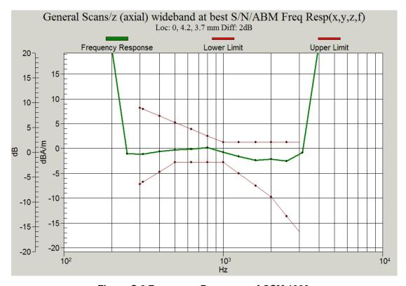
Figure C.2 Frequency Response of GSM 1900
