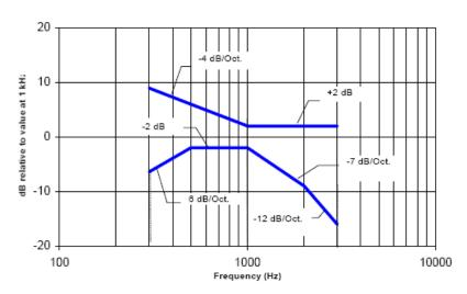
NOTE—Frequency response is between 300 Hz and 3000 Hz.
