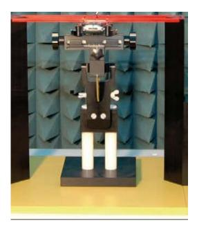
Figure 6.4 HAC Phantom & Device Holder
