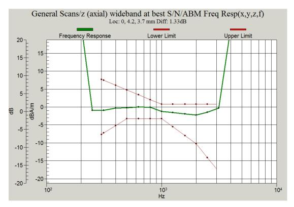
Figure C.1 Frequency Response of GSM 850
