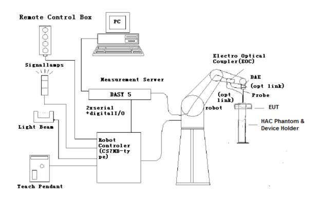
Figure 6.1 HAC Test Measurement Set-up
