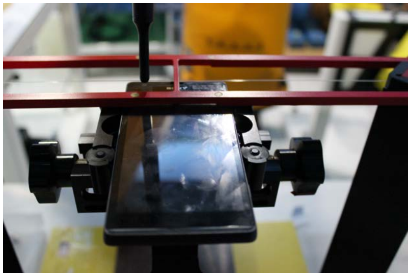
Picture 2: EUT Positioning for RF
