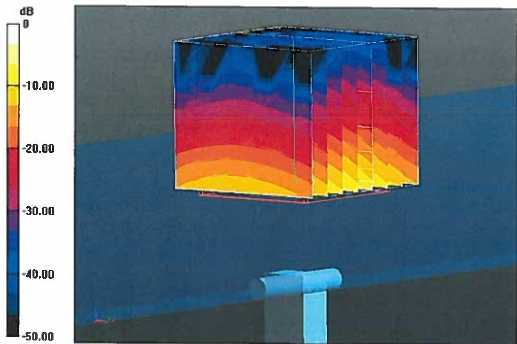
$0 \text{ dB} = 19.1 \text{ W/kg} = 12.81 \text{ dBW/kg}$
