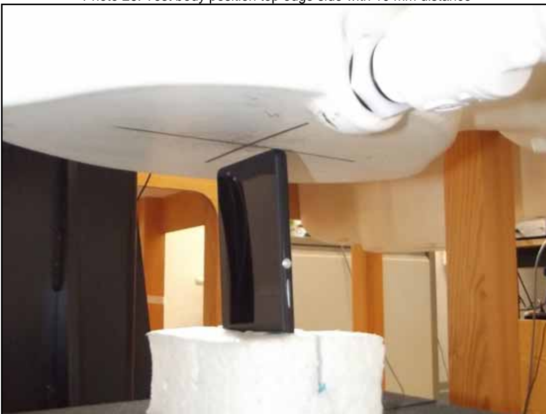
Photo 26: Test body position top edge side with 10 mm distance
