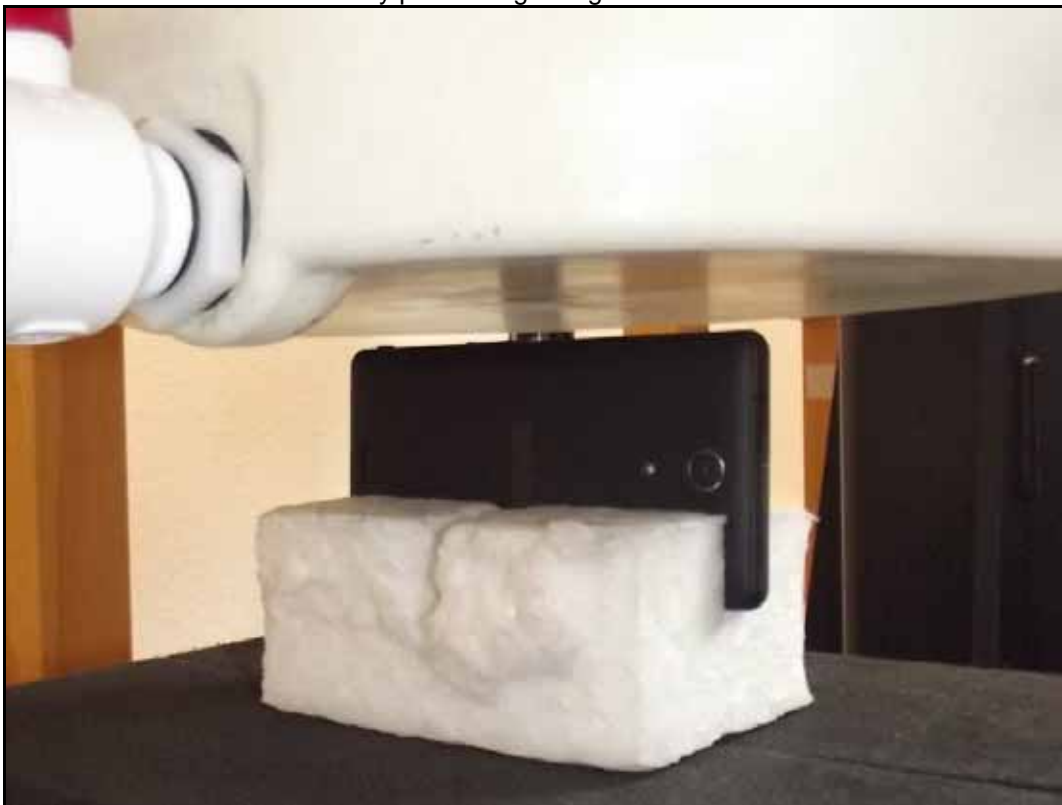
Photo 26: Test body position top edge side with 10 mm distance
