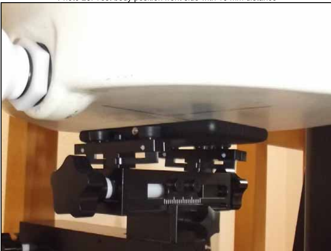
Photo 20: Test body position front side with 10 mm distance
