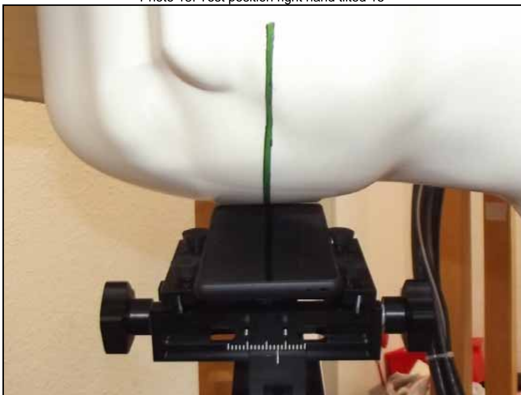
Photo 18: Test position right hand tilted 15°
