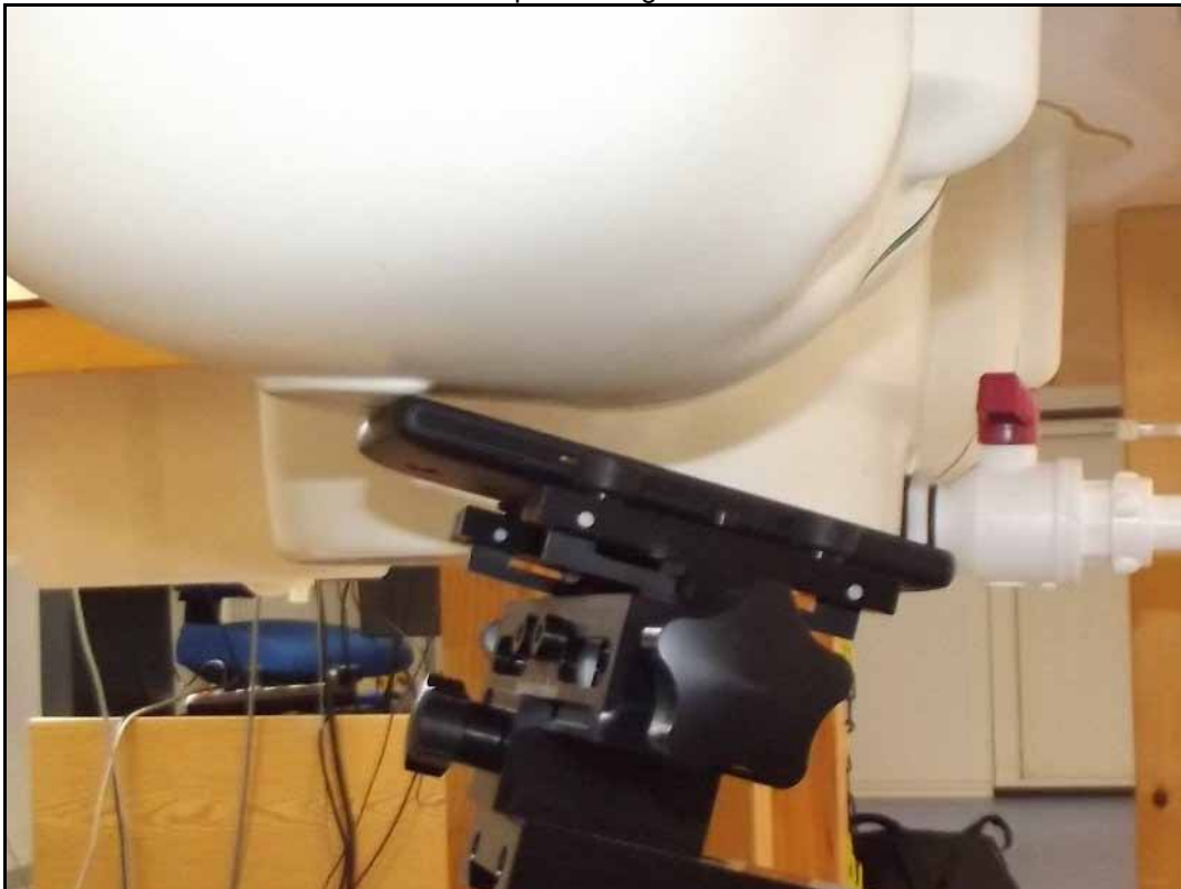
Photo 20: Test body position front side with 10 mm distance
