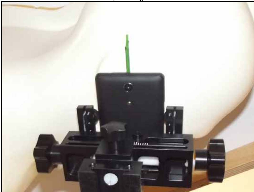
Photo 18: Test position right hand tilted 15°
