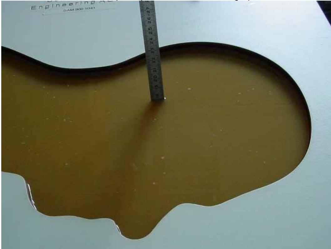
Photo 7: Liquid depth 5 GHz head simulating liquid
