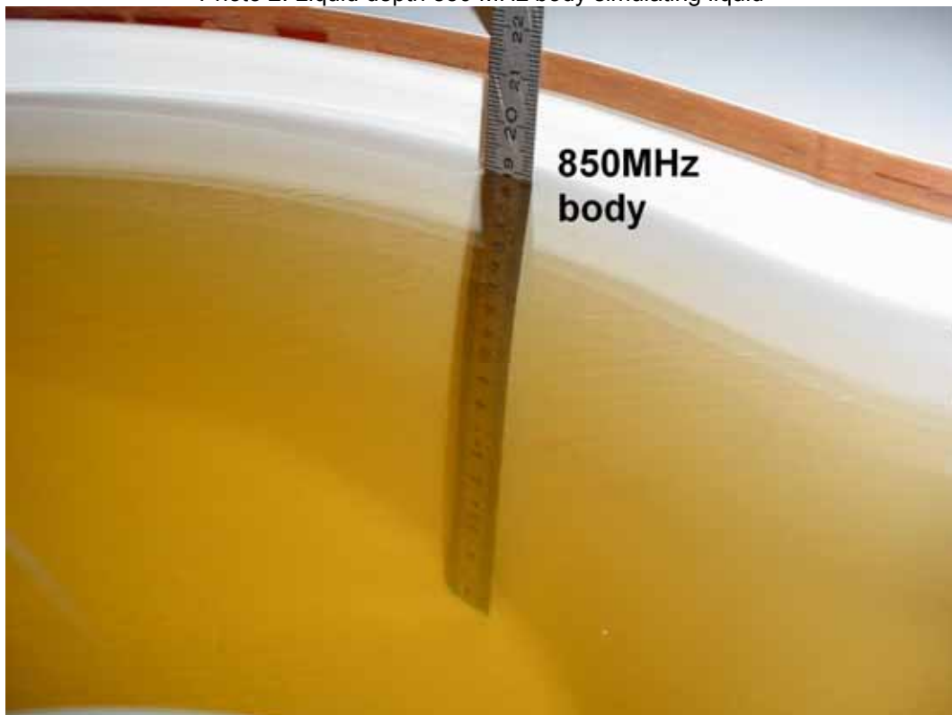
Photo 2: Liquid depth 850 MHz body simulating liquid
