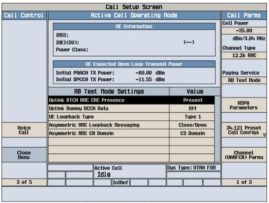
**Figure 7: RB Test Mode Settings**
