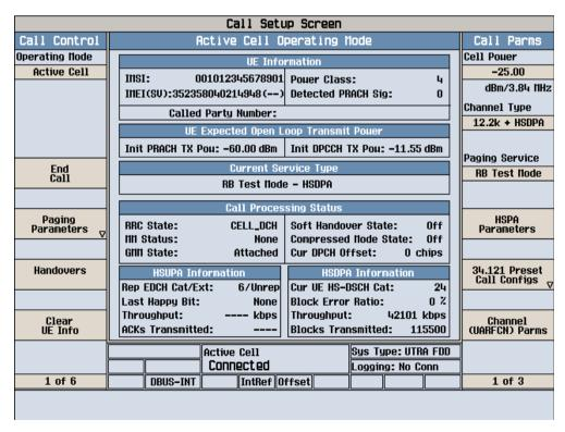
Now you can also check the connected DC-HSDPA downlink channel levels. Path: CALL SETUP->Call Control 2 of 6 -> Generator Info (F3) -> Additional Gen Info Screens (F1) -> DC-HSDPA DL Code Chan Info (F4).
