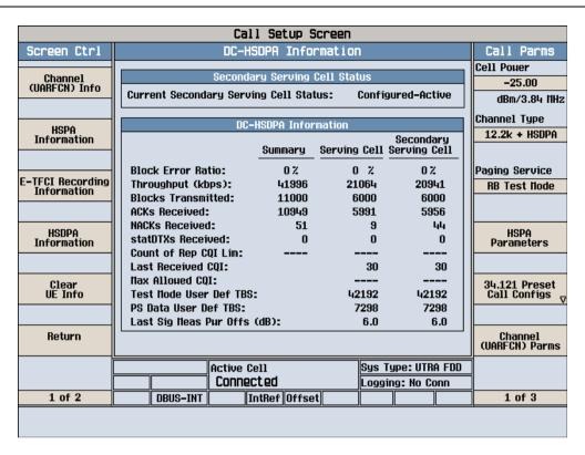
When DC-HSDPA is active, the HBLER measurement can also be used to perform receiver testing. 3GPP TS 34.121-1 sections 6.3C and 6.3D are supported and can be set up and tested as described in an appendix in another document, DC-HSDPA User Guide.
