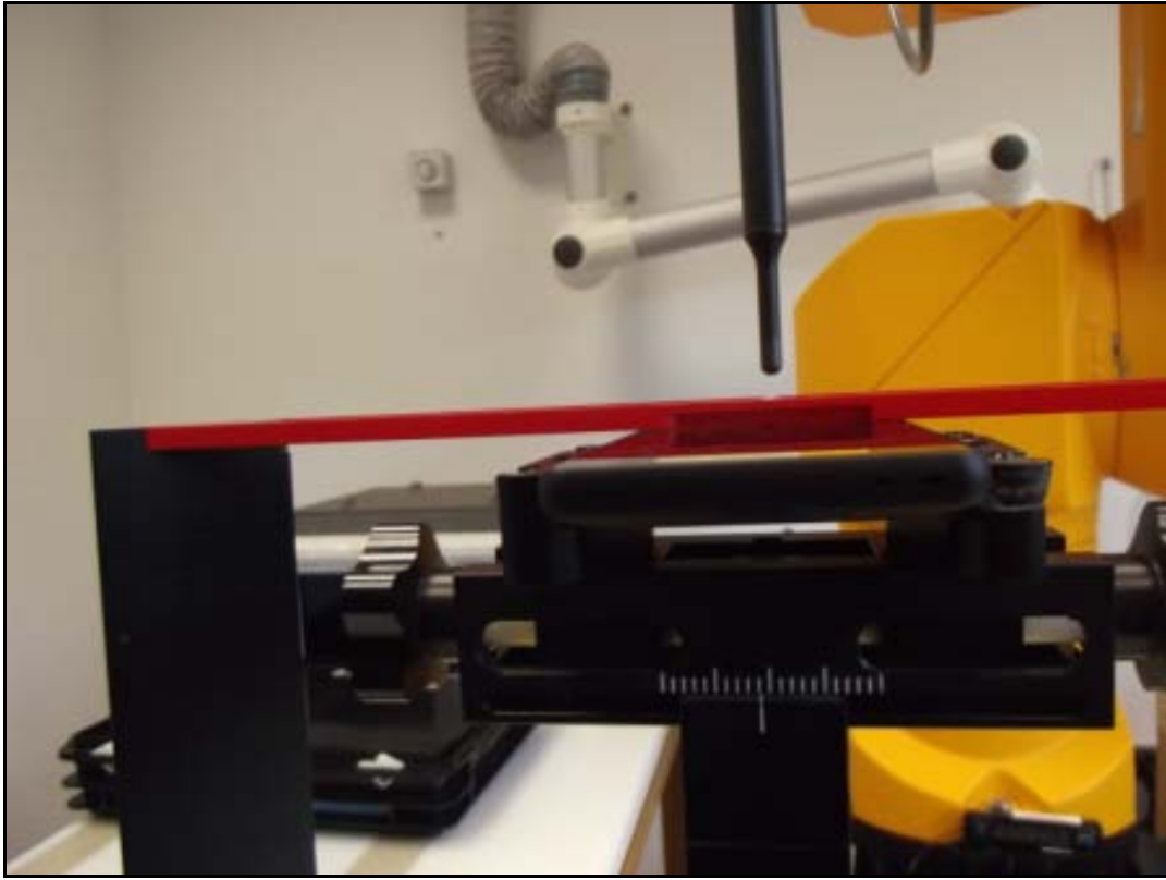
Photo 12: HAC system validation (shown with 835 MHz dipole)
