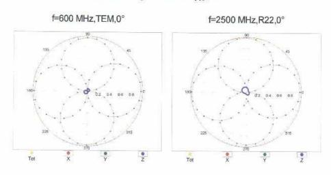
Receiving Pattern ( $\phi$ ),  $\vartheta = 0^{\circ}$
