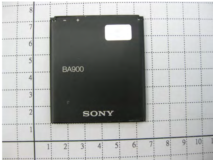
Fig.17 Front view of battery (Model No.: BA900, Supplier: SONY, Type No.: AB-0500)
