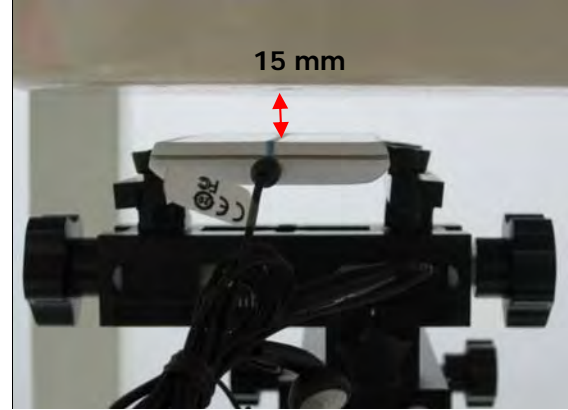
Fig.7 EUT front side with headset (MH410C) to flat phantom
