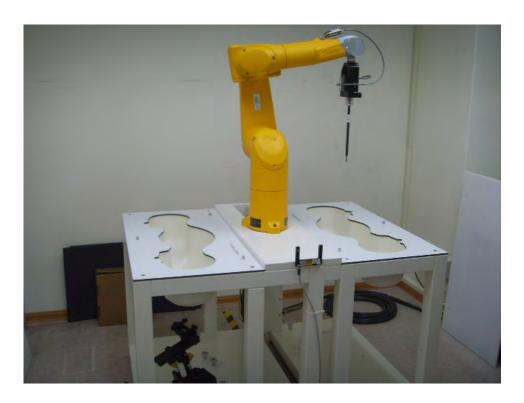
Fig.1 Photograph of the SAR measurement system
