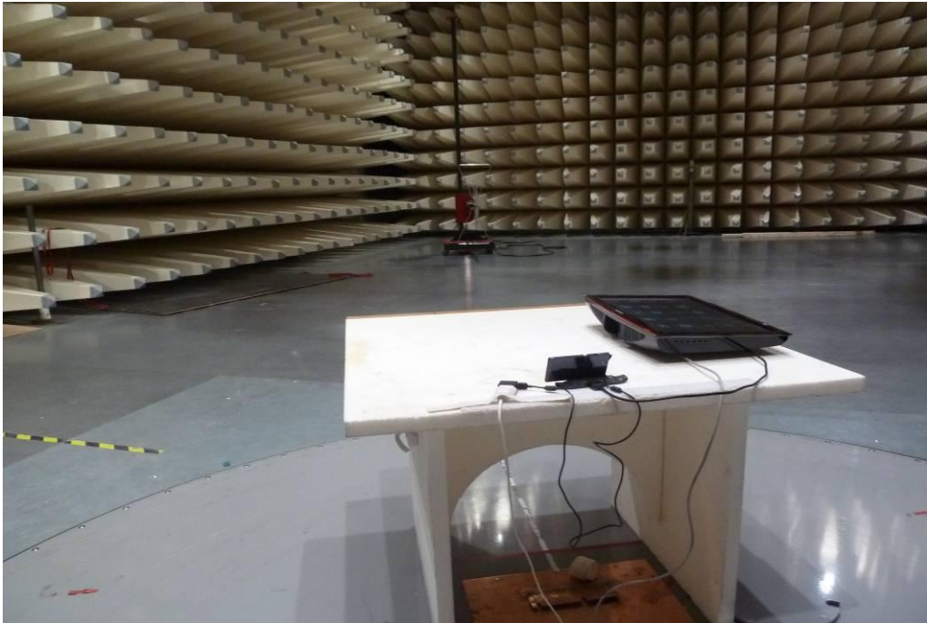
Photo 9: additional measurement HDMI connection via USB-cradle to monitor
