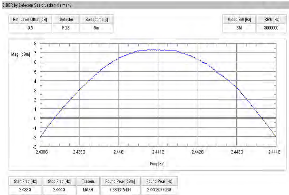
Plot 2: middle channel – 2441 MHz, GFSK modulation
