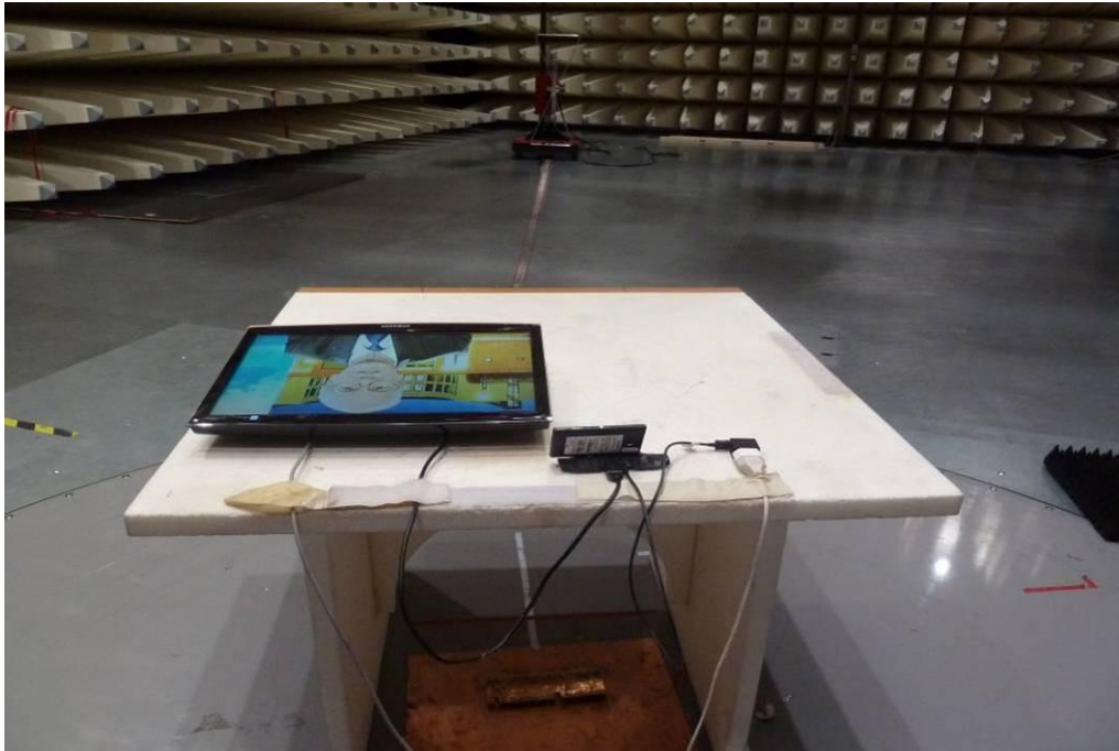
Photo 7: additional measurement with HDMI connection
