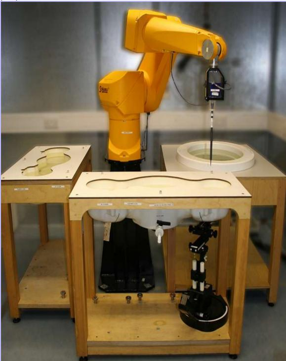
PHT/90893JD02/001: Test configuration for the measurement of Specific Absorption Rate (SAR)
