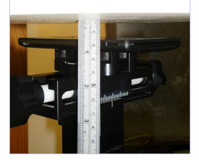
PHT/90893JD02/008: Back of EUT facing Phantom at 10mm
