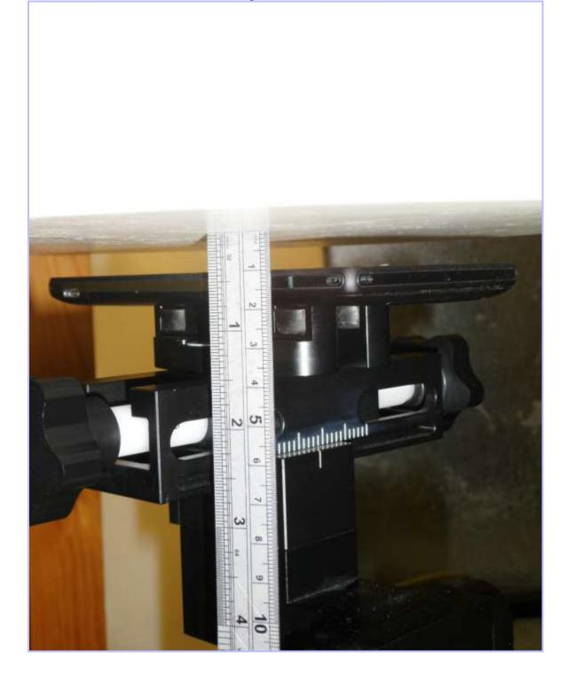
PHT/90893JD02/007: Front of EUT facing Phantom at 15mm
