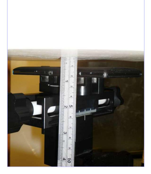
PHT/90893JD02/009: Back of EUT facing Phantom at 15mm
