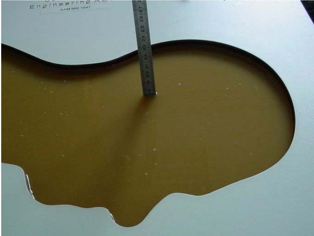
Photo 7: Liquid depth 5 GHz head simulating liquid
