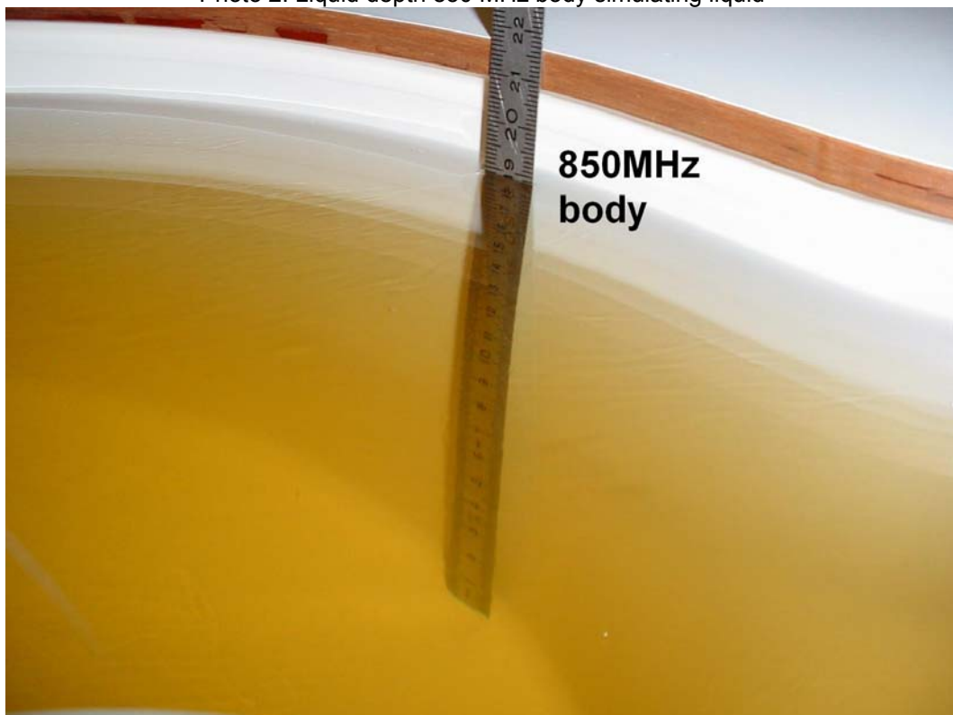
Photo 2: Liquid depth 850 MHz body simulating liquid
