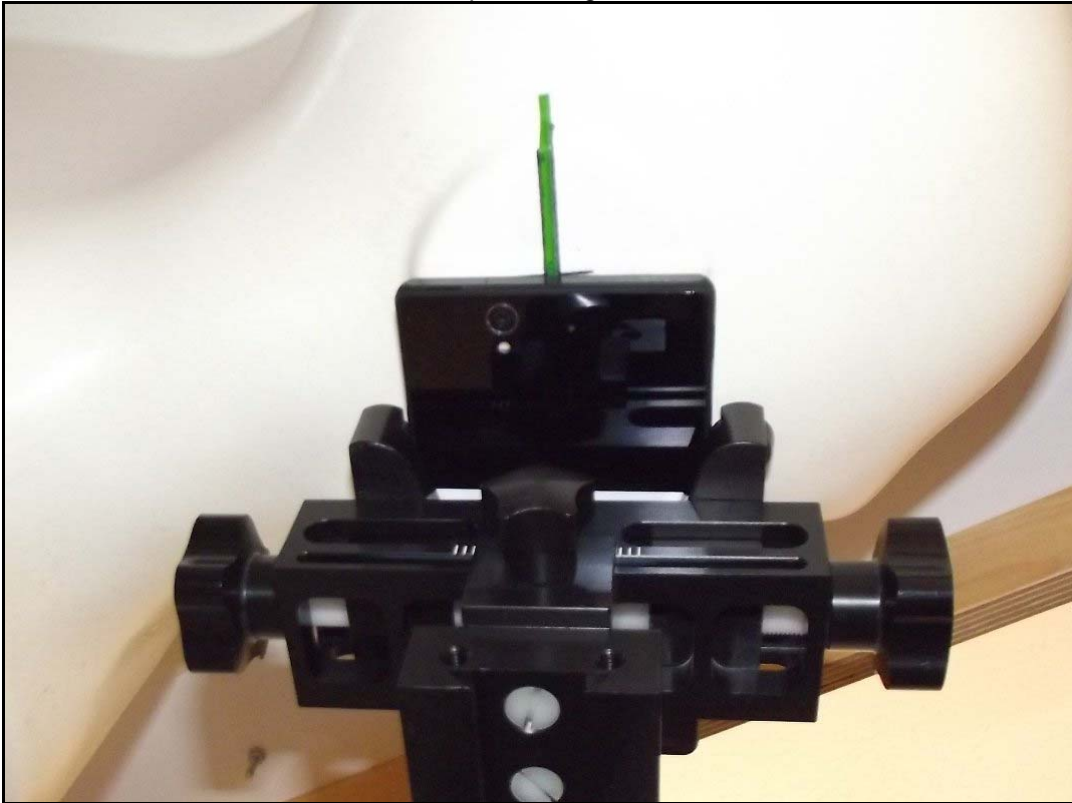
Photo 14: Test position right hand tilted 15°
