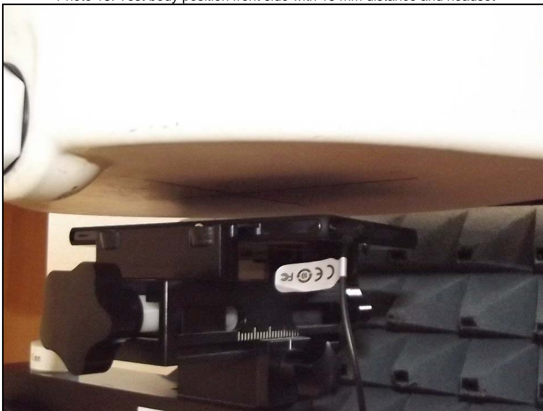
Photo 18: Test body position front side with 15 mm distance and headset
