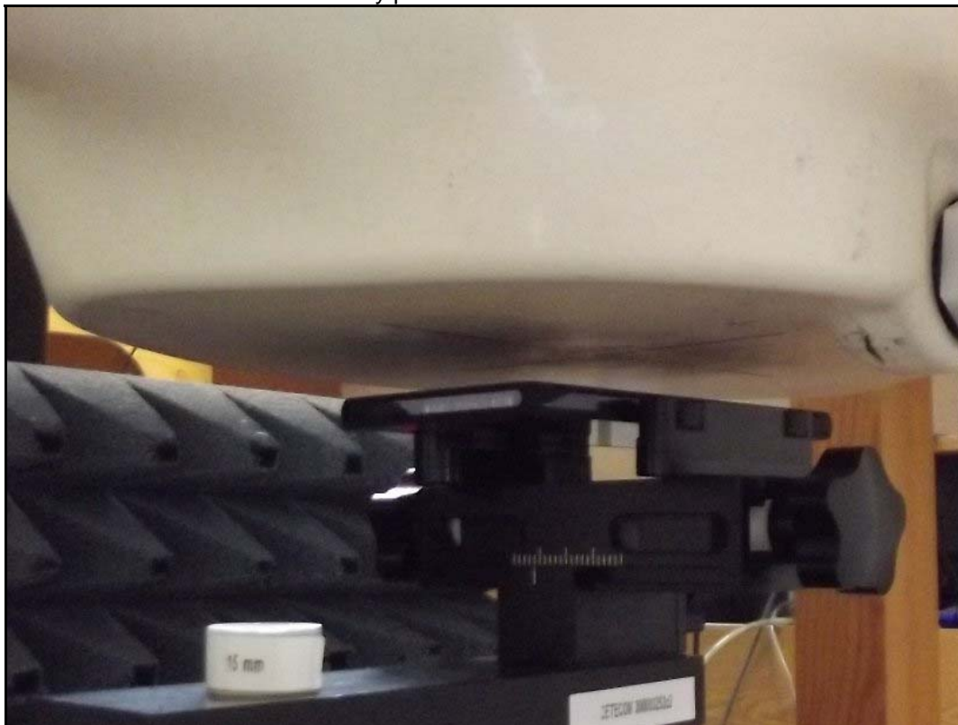
Photo 18: Test body position front side with 15 mm distance and headset
