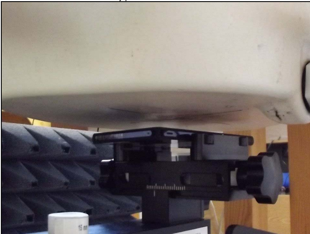
Photo 16: Test body position front side with 15 mm distance
