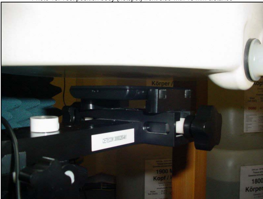
Photo 18: Test position body (hotspot) front side with 10 mm distance
