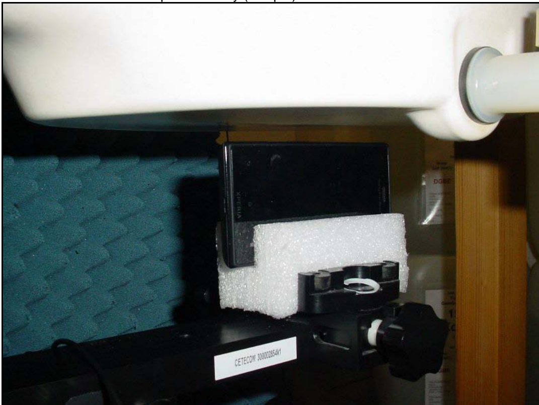
Photo 20: Test position body (hotspot) left side with 10 mm distance
