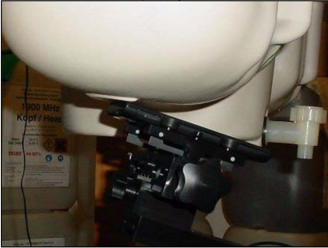
Photo 16: Test position body worn front side with 15 mm distance
