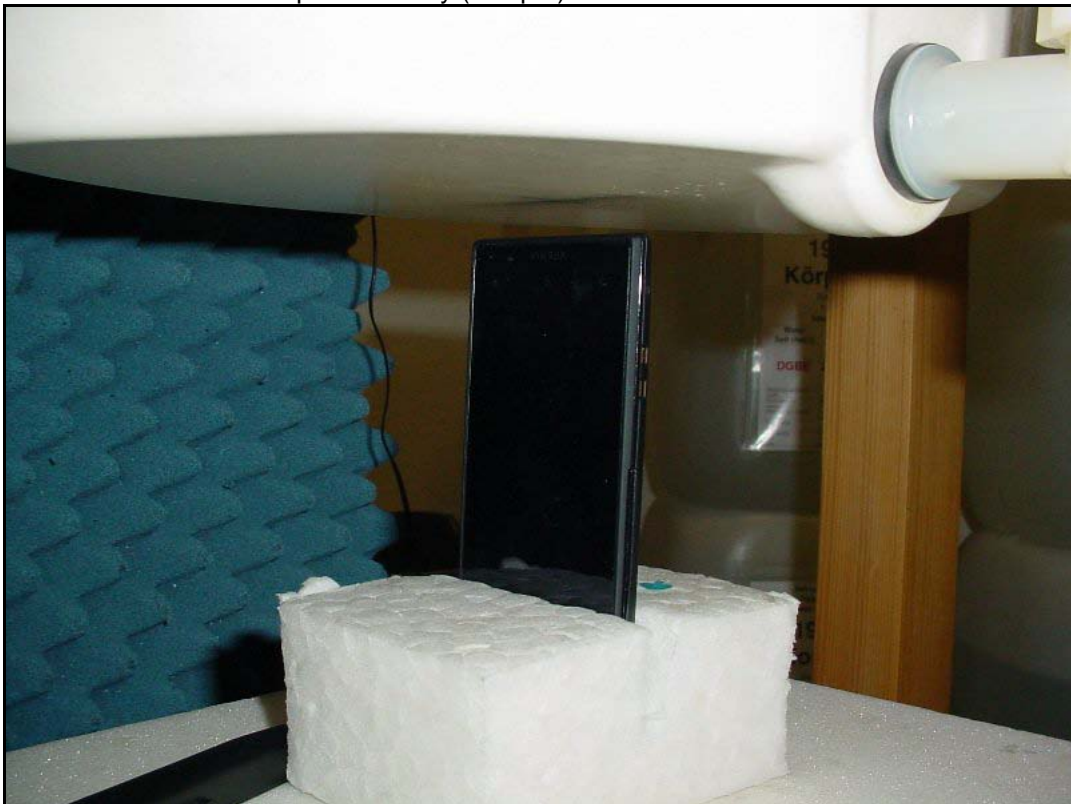
Photo 22: Test position body (hotspot) bottom side with 10 mm distance
