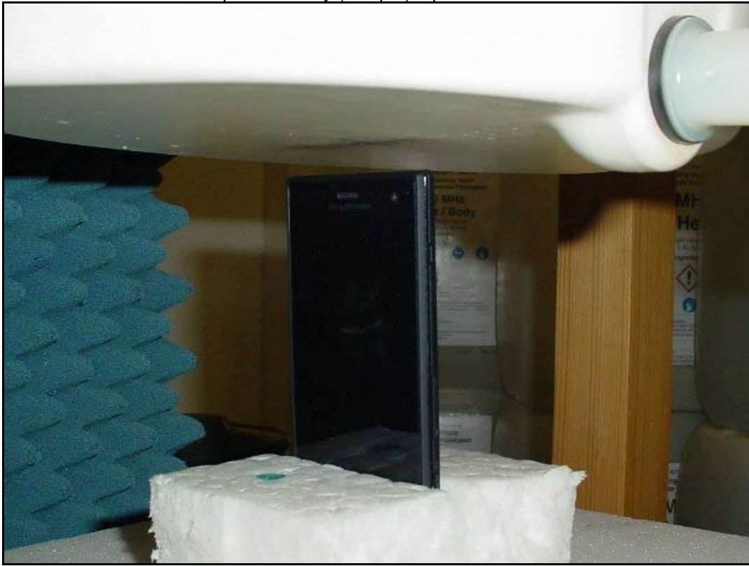
Photo 23: Test position body (hotspot) top side with 10 mm distance
