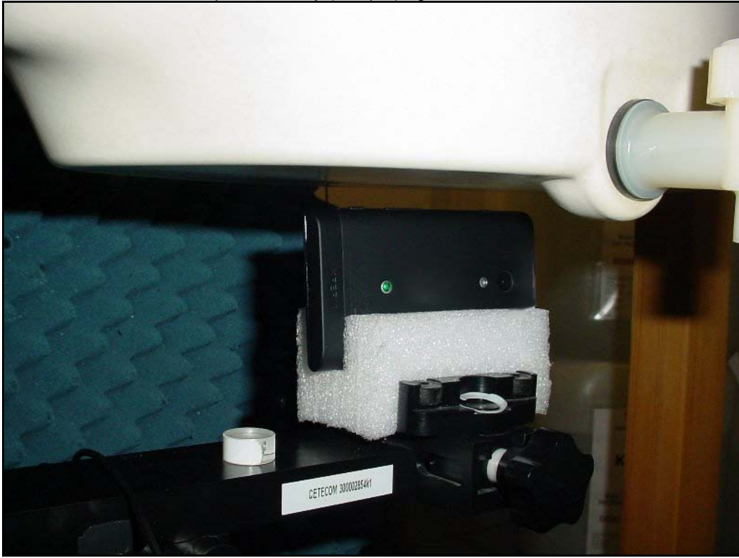
Photo 22: Test position body (hotspot) bottom side with 10 mm distance
