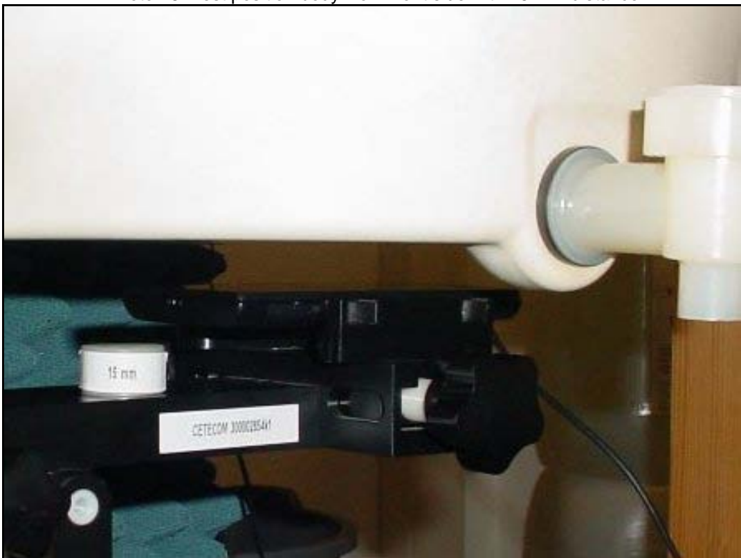
Photo 16: Test position body worn front side with 15 mm distance
