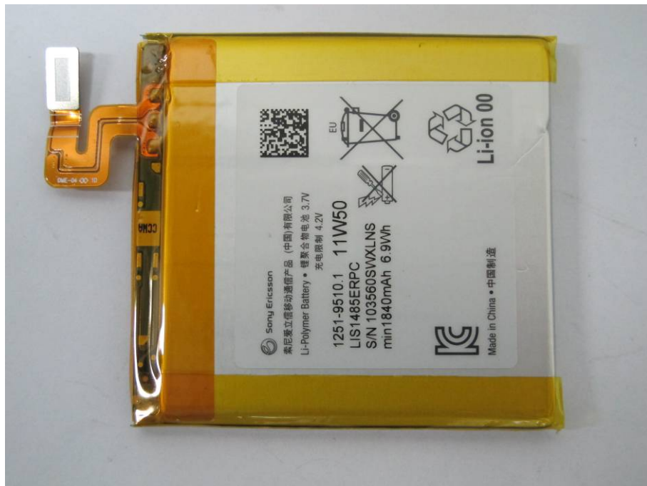
Inbuilt Li-Polymer Battery
