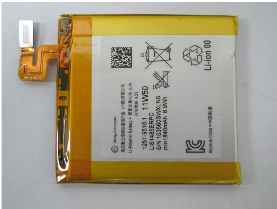
Inbuilt Li-Polymer Battery
