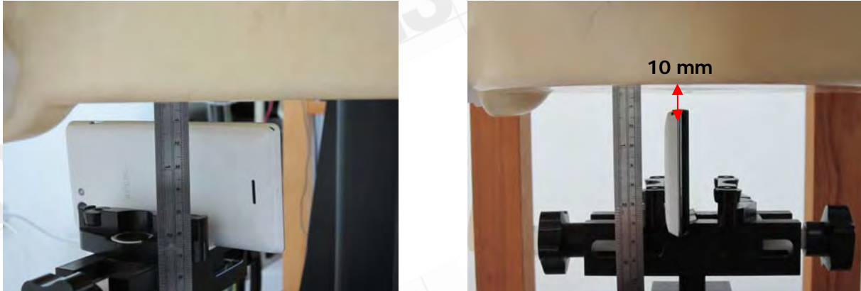
Fig.15 EUT left to flat phantom
