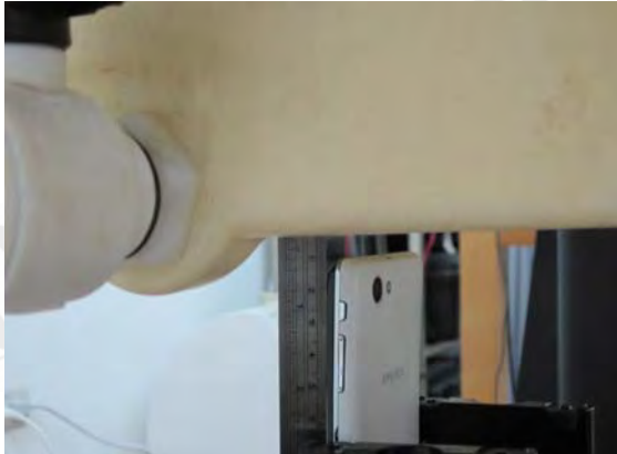
Fig.12 EUT top to flat phantom
