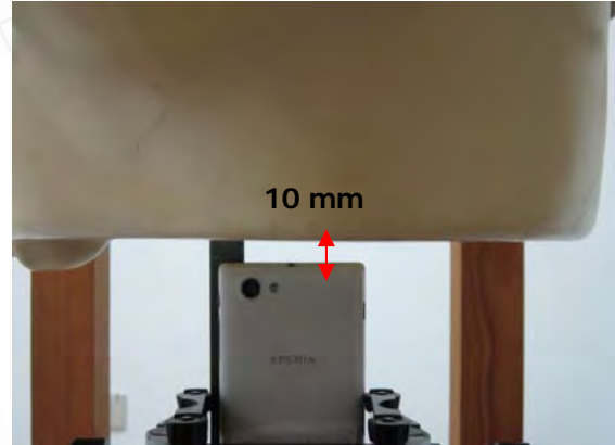
Fig.12 EUT top to flat phantom
