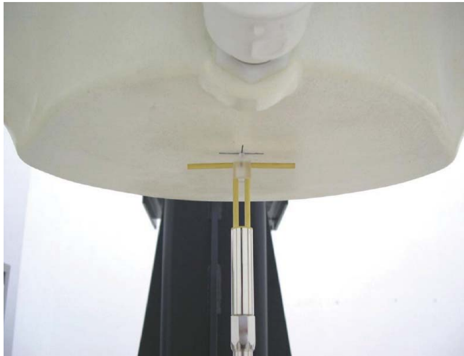
Picture 19 Photo of Dipole Setup
