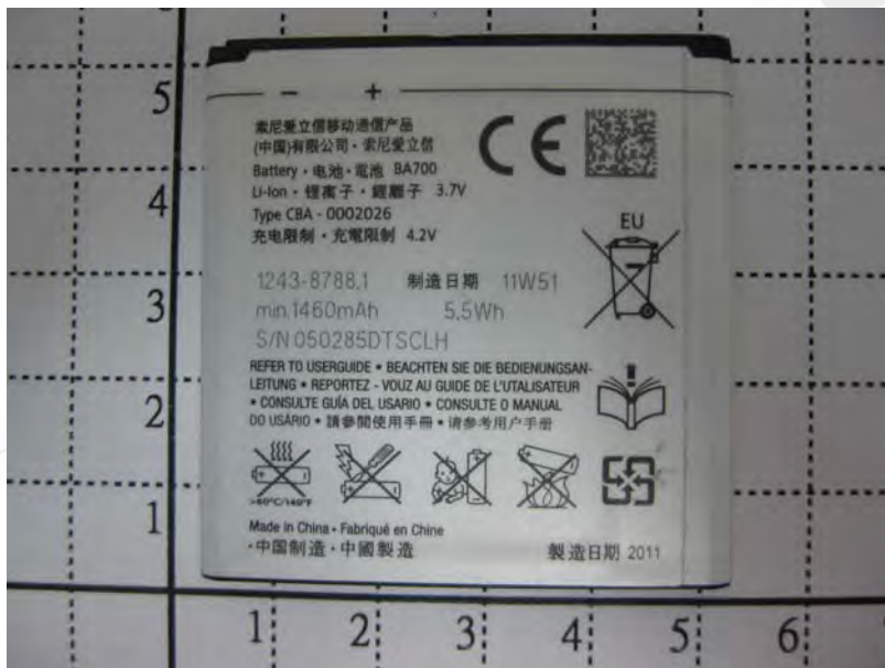
Fig.21 Back view of 2 nd Battery (Model No.: BA700, Supplier: Samsung, Type No.: CBA-0002026)
