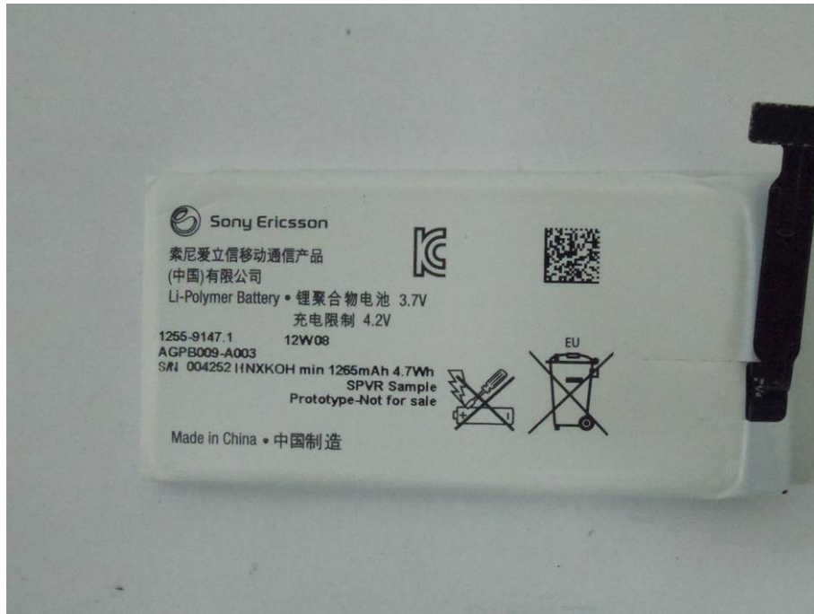
Inbuilt Li-Polymer Battery
