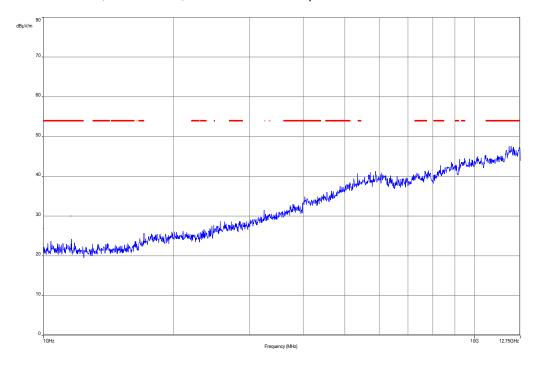
Carrier suppressed with a 2.4 GHz-band rejection filter.
