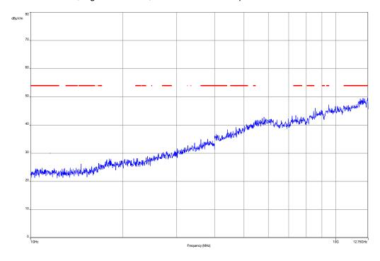
Carrier suppressed with a 2.4 GHz-band rejection filter.
