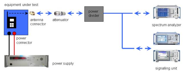
Picture 2: Diagram conducted measurements
