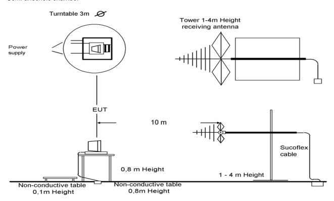
Picture 1: Diagram radiated measurements
