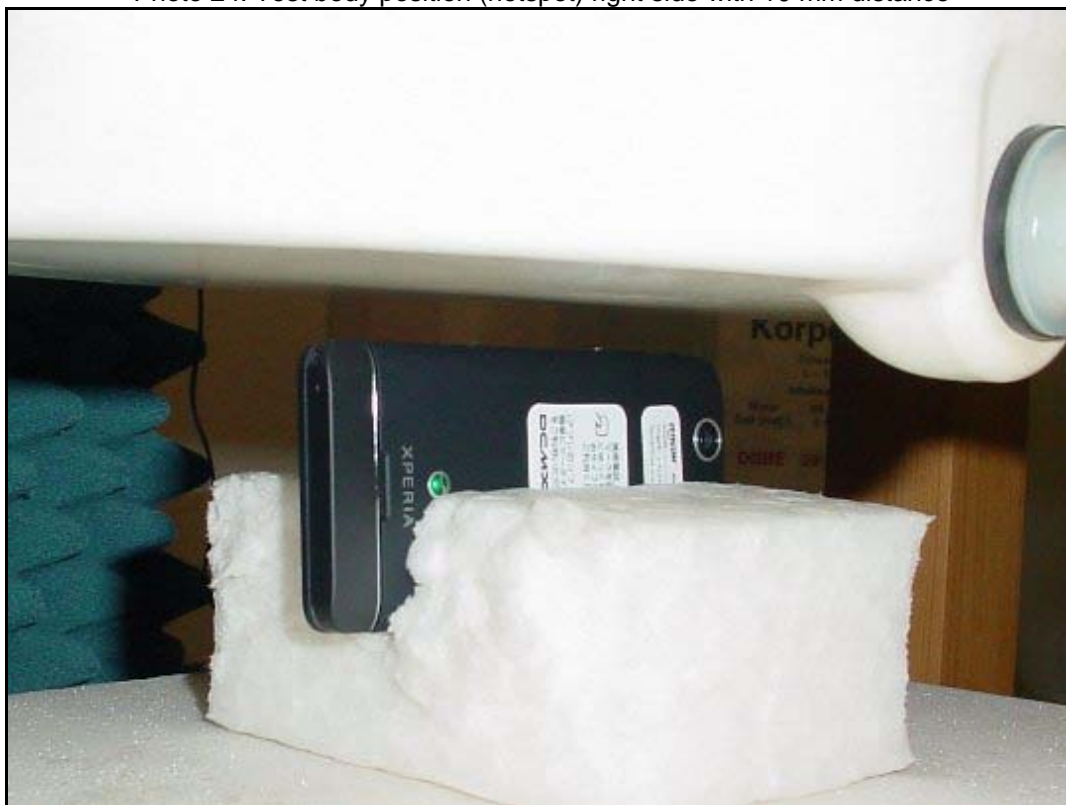
Photo 24: Test body position (hotspot) right side with 10 mm distance
