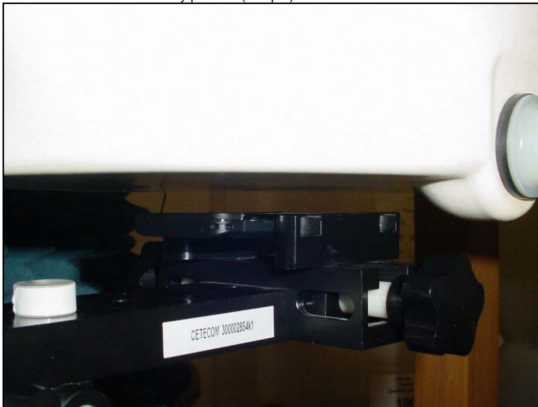
Photo 22: Test body position (hotspot) rear side with 10 mm distance
