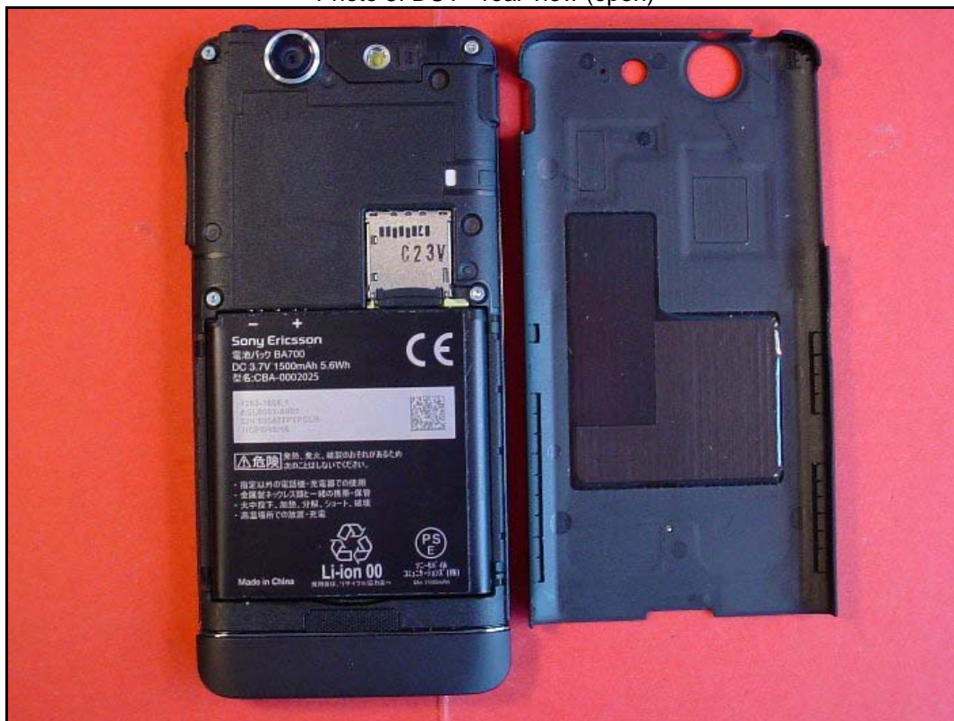
Photo 6: DUT - rear view (open) without battery
