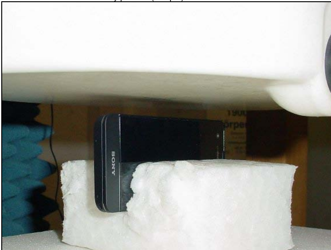
Photo 24: Test body position (hotspot) right side with 10 mm distance
