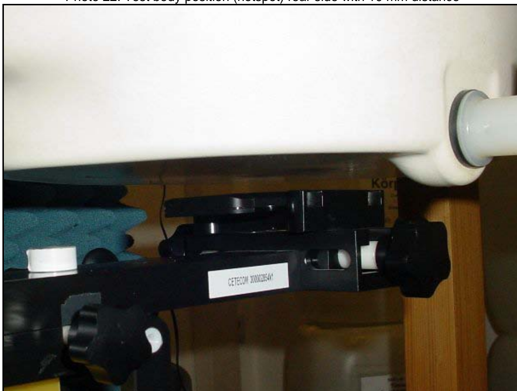
Photo 22: Test body position (hotspot) rear side with 10 mm distance
