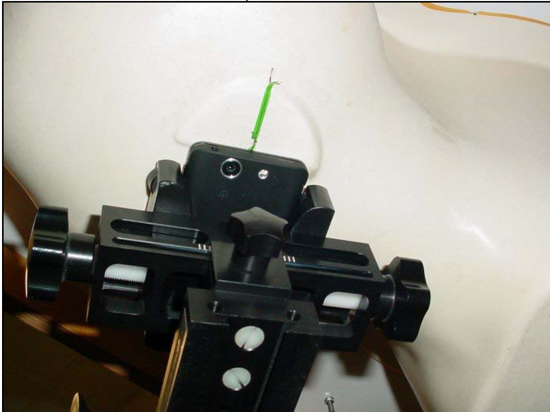
Photo 12: Test position left hand tilted 15°
