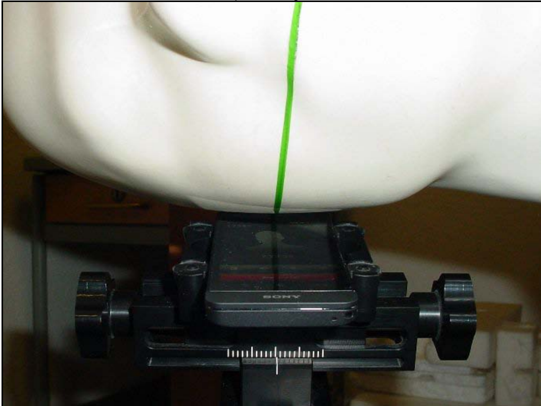
Photo 18: Test position right hand tilted 15°
