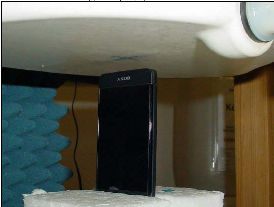
Photo 26: Test body position (hotspot) top side with 10 mm distance
