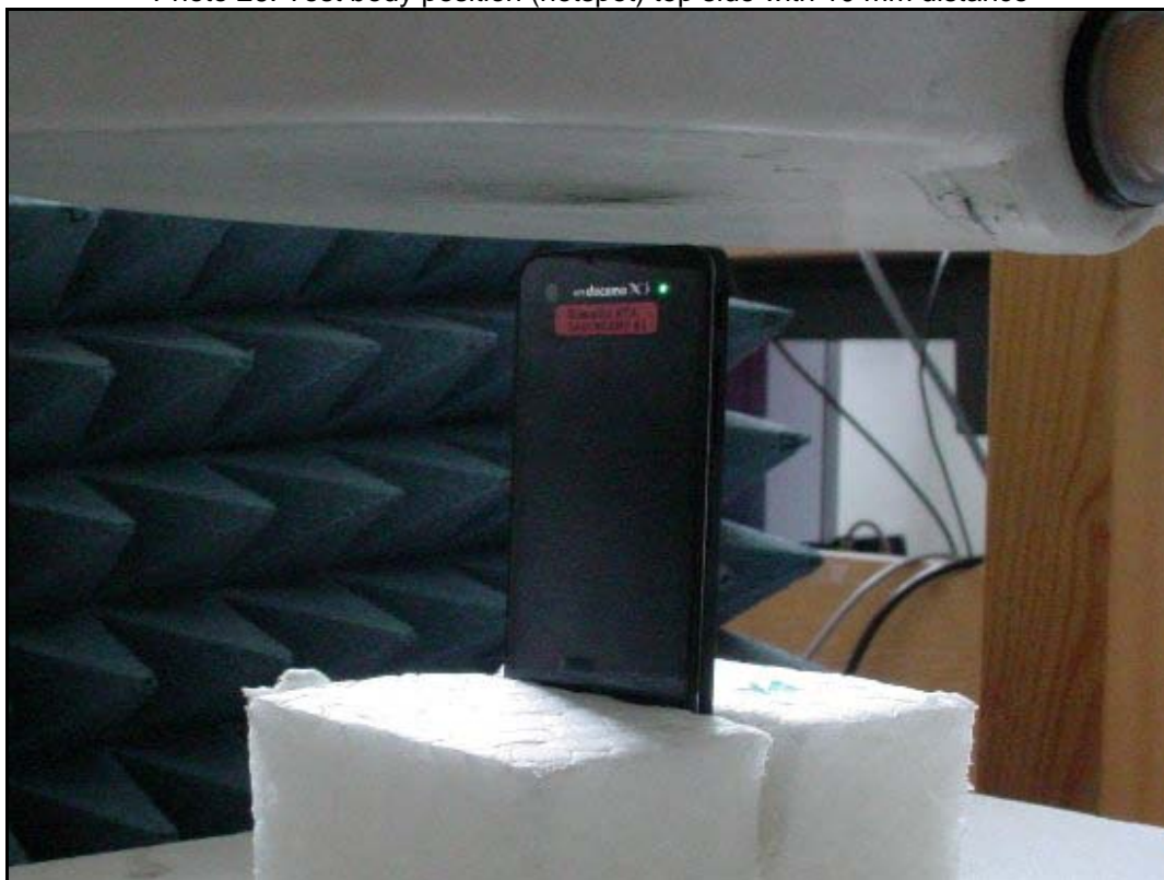
Photo 26: Test body position (hotspot) top side with 10 mm distance
