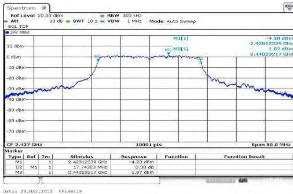
Plot 2: TX mode, middle channel, 6 dB bandwidth
