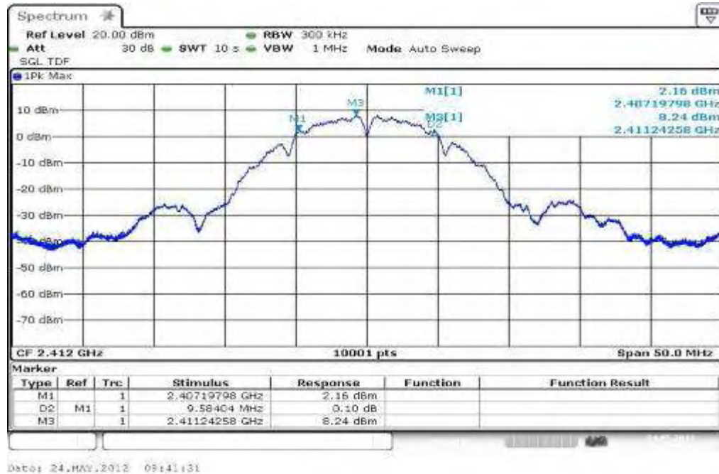
Plot 1: TX mode, lowest channel, 6 dB bandwidth
