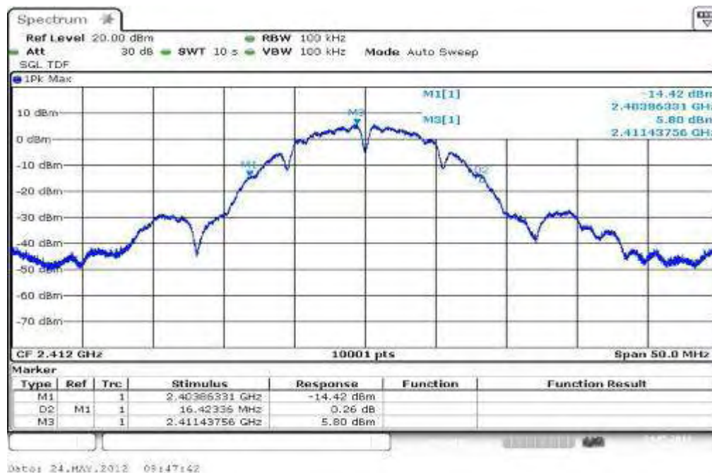
Plot 1: TX mode, lowest channel, 20 dB bandwidth
