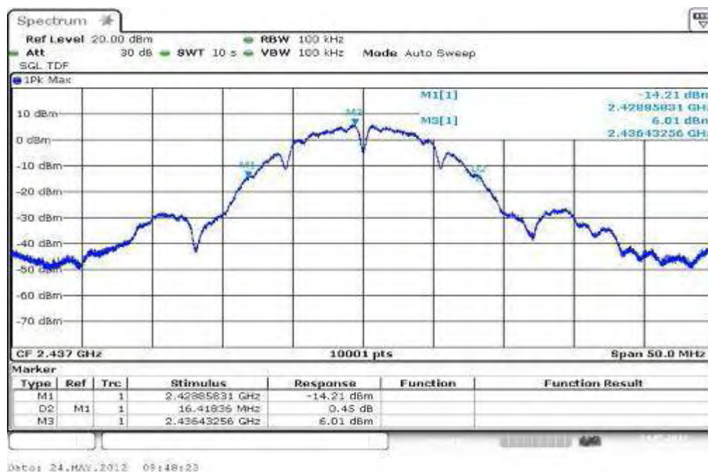
Plot 2: TX mode, middle channel, 20 dB bandwidth
