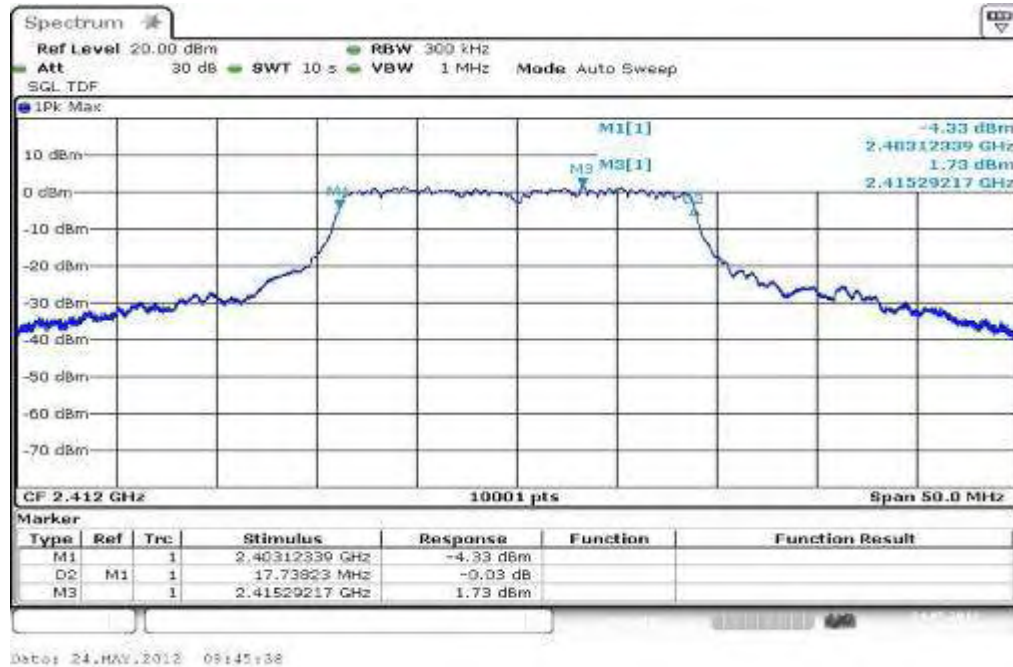
Plot 1: TX mode, lowest channel, 6 dB bandwidth
