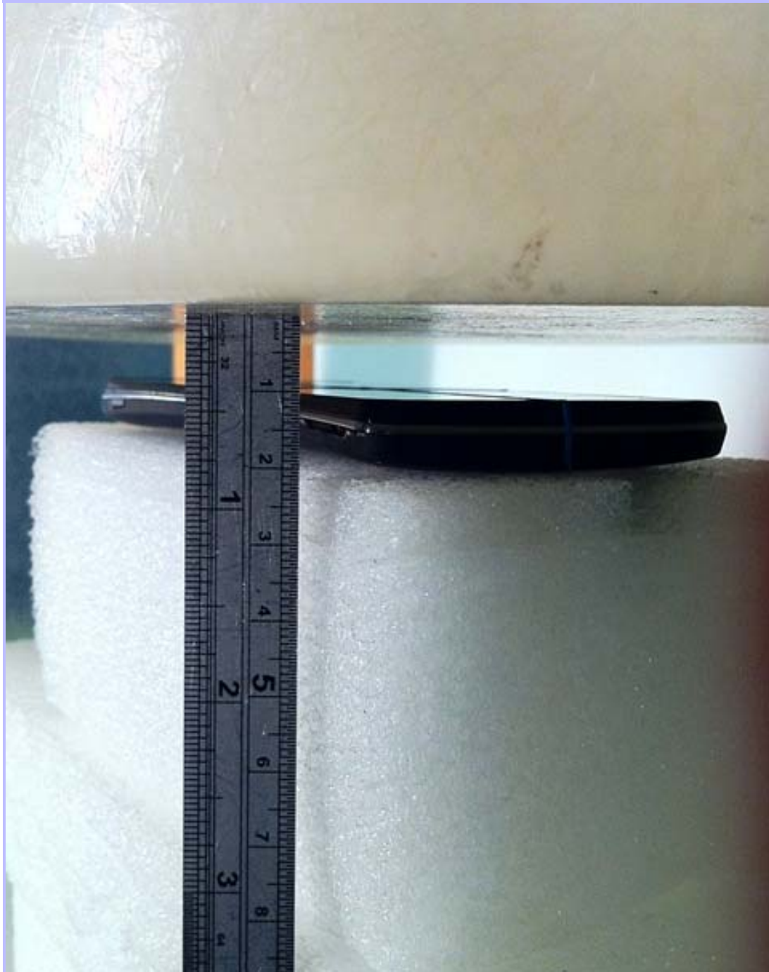
PHT/86599JD02/006: Front of EUT Facing Phantom at 10mm separation
