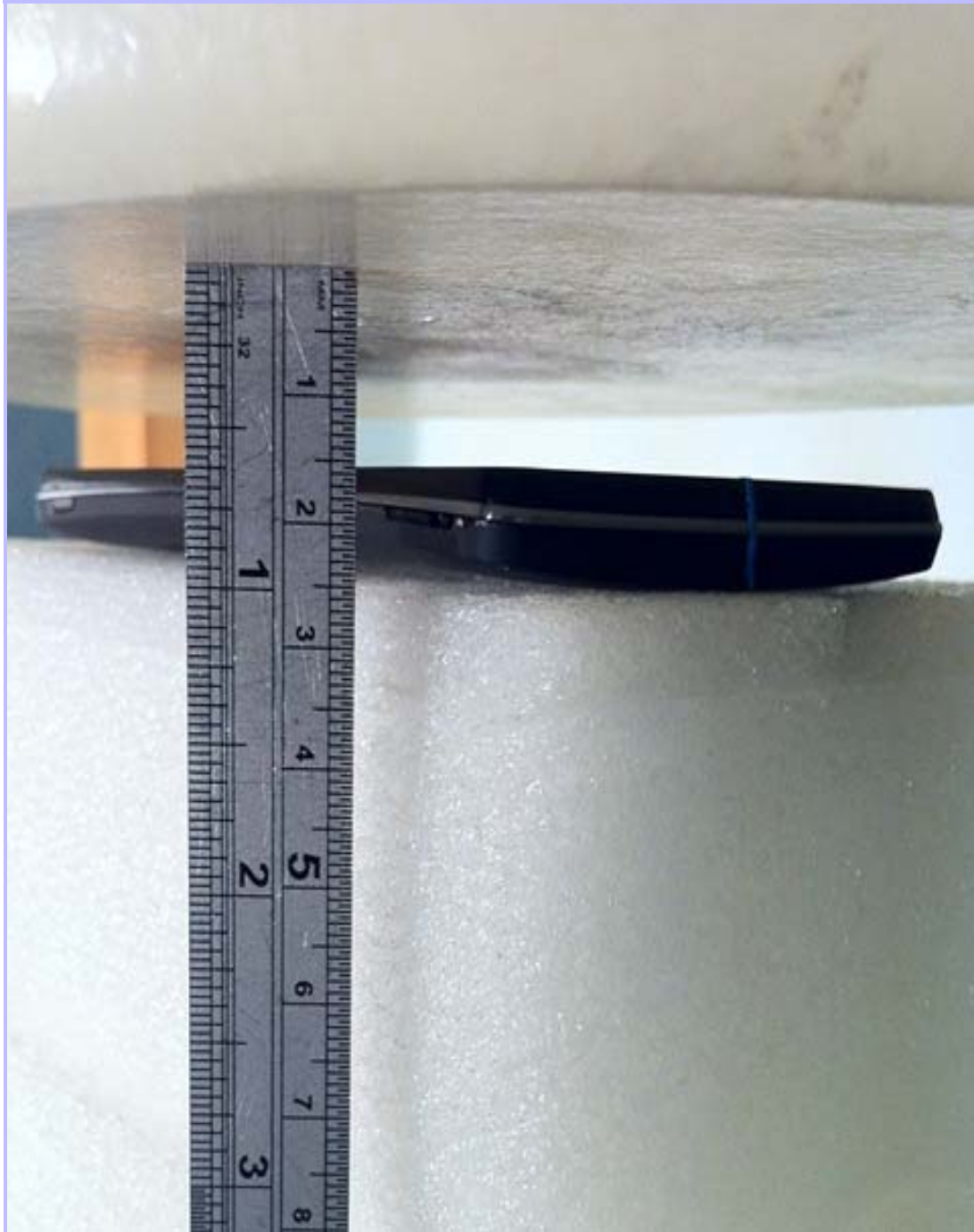
PHT/86599JD02/007: Front of EUT Facing Phantom at 15mm separation
