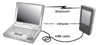
To synchronize, connect your phone to the computer using a USB, Bluetooth or infrared connection.
