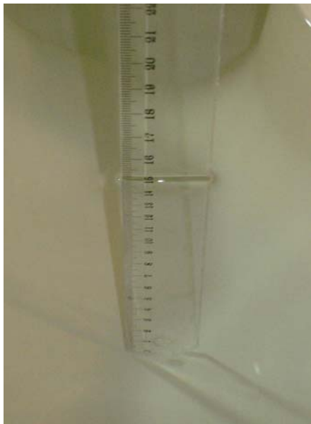
Measured level of 1900 MHz head tissue simulating liquid in phantom
