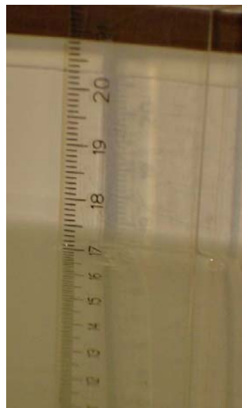
Measured level of 1900 MHz muscle tissue simulating liquid in phantom
