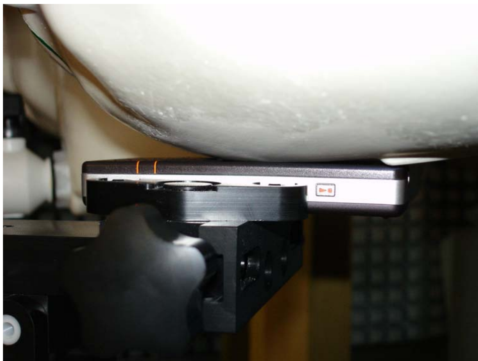
(a) Device on head phantom in the cheek position.
