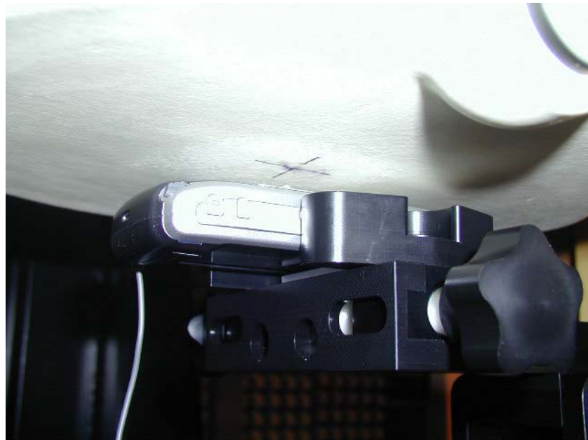
(d) Device on flat section of the phantom with the stereo headset. The separation was 15 mm between the device and the tissue simulating liquid.
