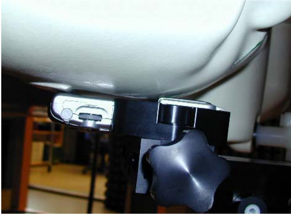
(a) Device on head phantom in the cheek position with the flip closed.
