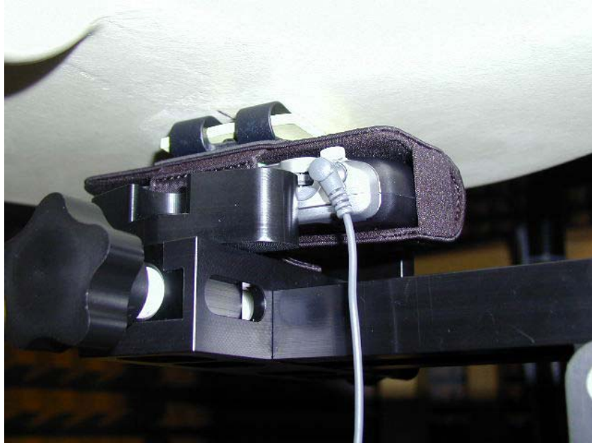
(c) Device on flat section of the phantom with the carry case and the stereo headset. The clip was opened 3 mm with a piece of paper.
