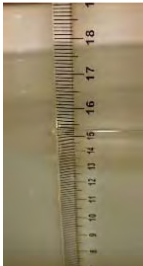
Measured level (153 mm, head section) of 1900 MHz head tissue simulating liquid in phantom.
