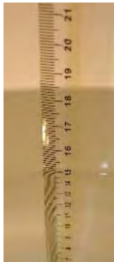
Measured level (152 mm, flat section) of 1900 MHz muscle tissue simulating liquid in phantom.
