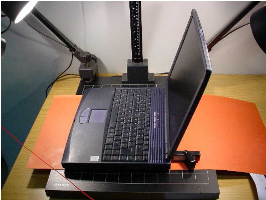
Photo 16: Laptop Sony Vaio with DUT (vertical slot)
