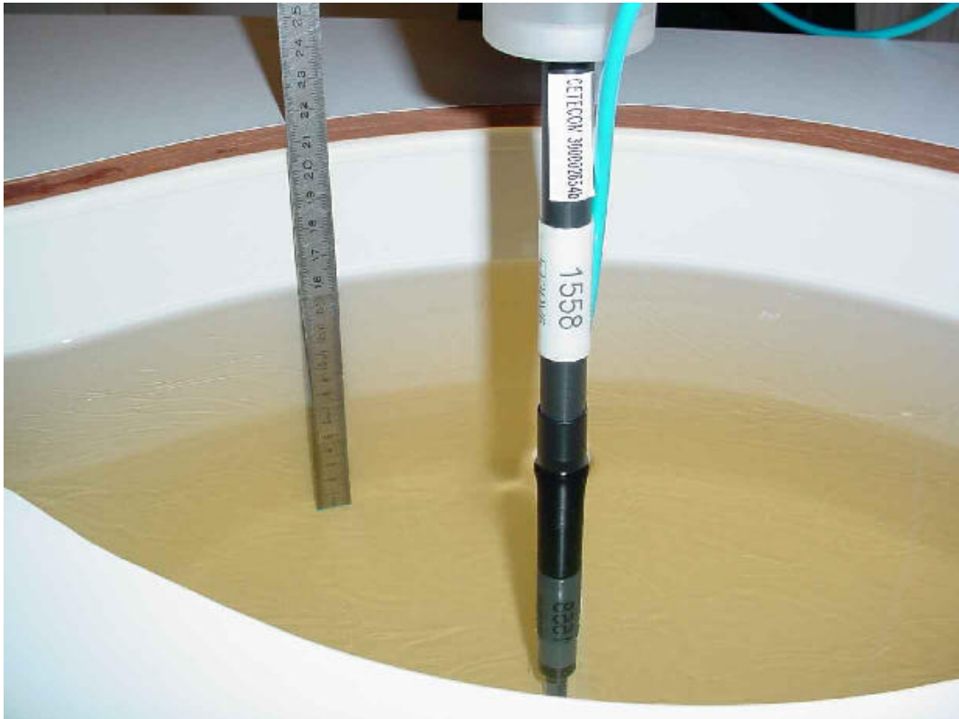
Photo 33: Liquid depth 1900 MHz body simulating liquid
