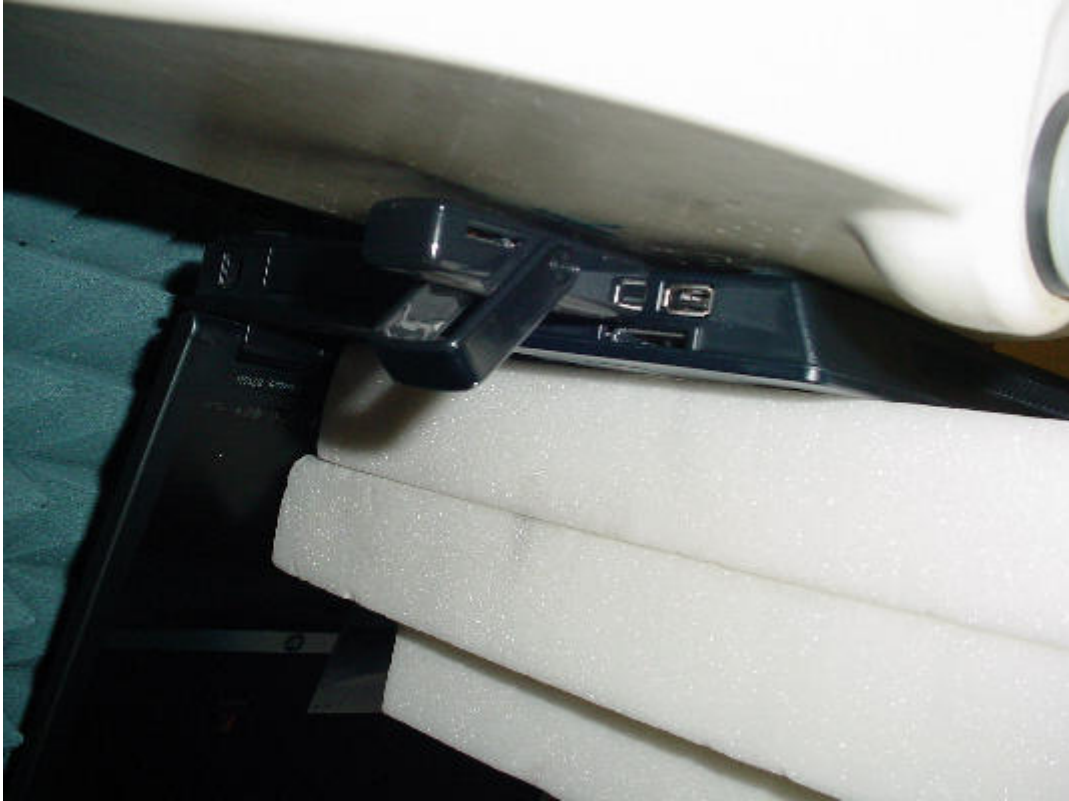
Photo 26: test position underside with horizontal slot (3 mm distance) 120° angle
