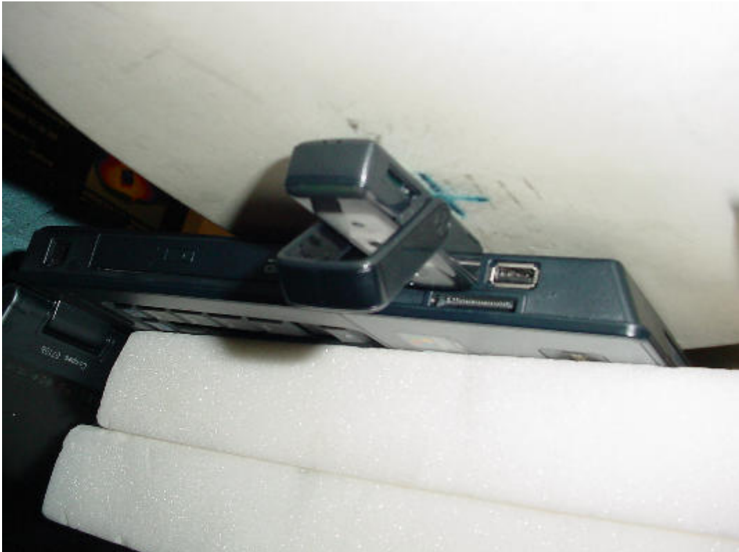
Photo 26: test position underside with horizontal slot (3 mm distance) 120° angle
