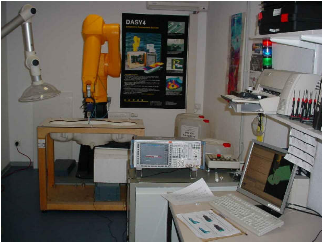
Photo 2: Measurement System DASY 4
