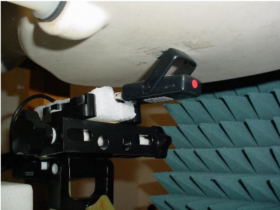
Photo 30: test position top side (0 mm distance)
