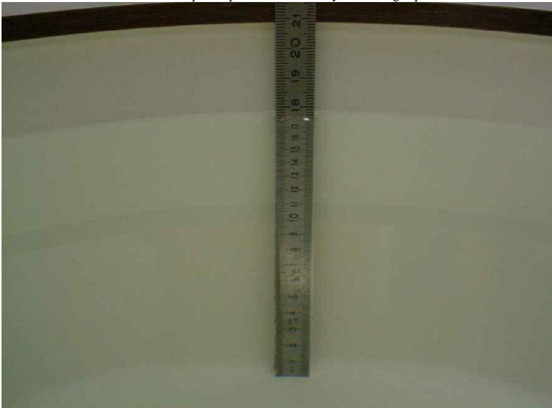
Photo 33: Liquid depth 1900 MHz body simulating liquid
