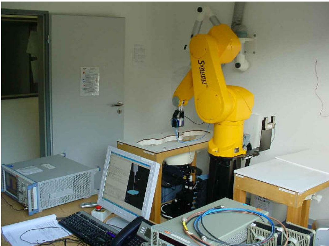
Photo 2: Measurement System DASY 4
