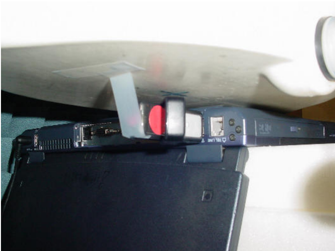
Photo 28: test position left side with vertical slot (5 mm distance)
