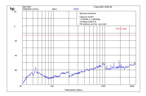
f < 1 GHz : RBW/VBW: 100 kHz Carrier suppressed with a rejection filter  $\mathrm{f} \geq 1\mathrm{GHz}:\mathrm{RBW} \slash \mathrm{VBW} \slash \mathrm{MHz}$
