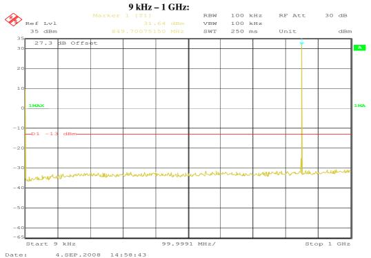
The peak at the beginning of the Plot is the LO from the measuring spectrum Analyzer and not from the EUT.
