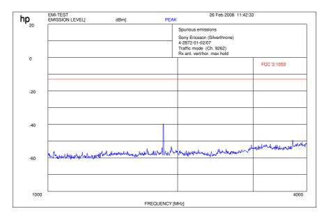
RBW / VBW 1 MHz Carrier suppressed with a rejection filter
