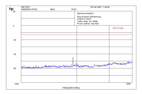
f > 1 GHz : RBW / VBW 1 MHz Carrier suppressed with a rejection filter
