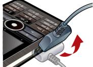
Remove the charger by tilting the plug • upwards.
