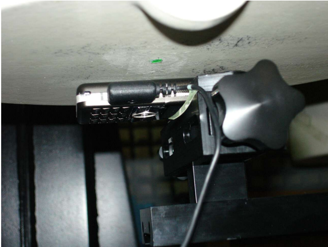
(c) Device on flat section of the phantom. The separation was 15 mm between the device and the flat phantom.
