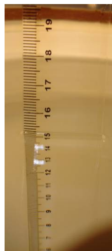
Measured level (153 mm, head section) of 2450 MHz head tissue simulating liquid in phantom
