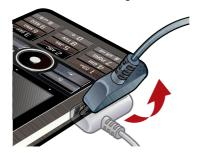
Remove the charger by tilting the plug upwards.
