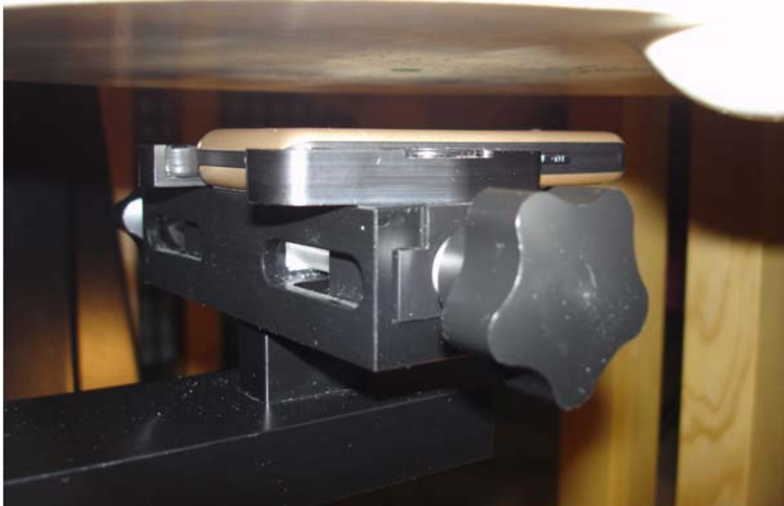
(c) Device on flat section of the phantom. The separation was 15 mm between the device and the flat phantom.
