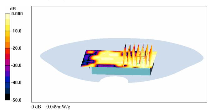
(k) Maximum SAR Distribution for EUT in WLAN mode measured with the back of the phone facing the flat section of phantom.
