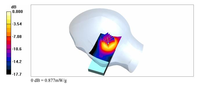
(b) SAR Distribution for EUT in GSM1900 mode measured against the right hand side phantom for the tilt phone position.
