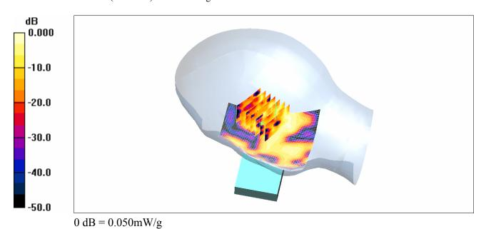
(h) SAR Distribution for EUT in WLAN mode measured against the right hand side phantom for the tilt phone position.
