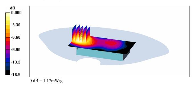
(e) Maximum SAR Distribution for EUT in GSM1900 mode measured with the back of the phone facing the flat section of phantom.
