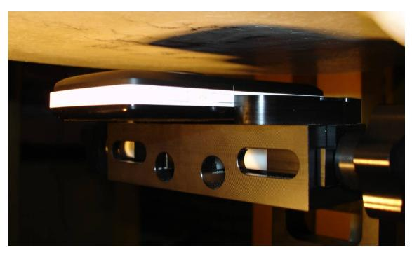
(c) Device on flat section of the phantom. The separation was 15 mm between the device and the flat phantom.  $\,$
