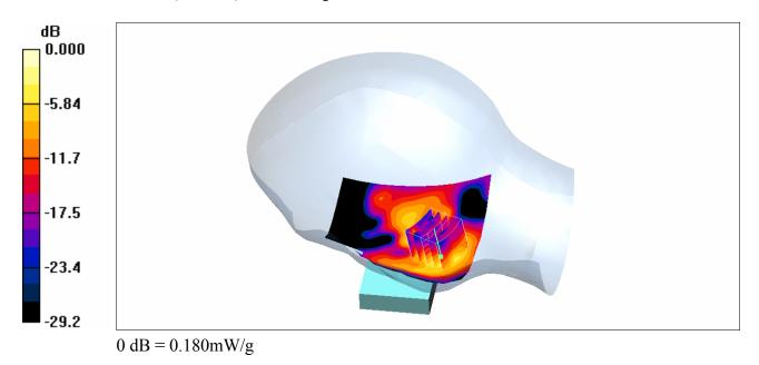
(g) Maximum SAR Distribution for EUT in WLAN mode measured against the right hand side phantom for the cheek phone position.
