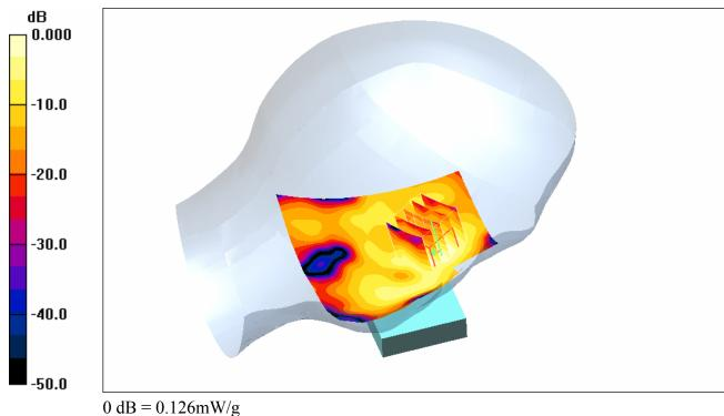
(i) SAR Distribution for EUT in WLAN mode measured against the left hand side phantom for the cheek phone position.
