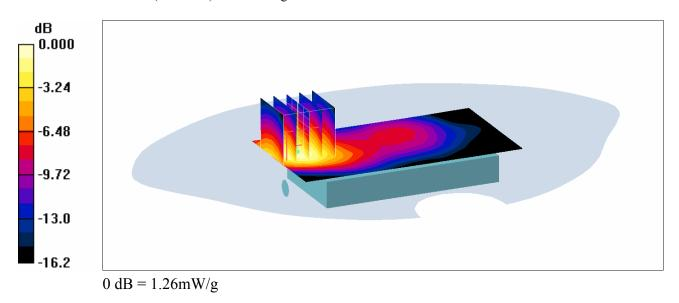
(f) Maximum SAR Distribution for EUT in GPRS(2Tx)1900 mode measured with the back of the phone facing the flat section of phantom.
