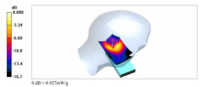
(d) SAR Distribution for EUT in GSM1900 mode measured against the left hand side phantom for the tilt phone position.
