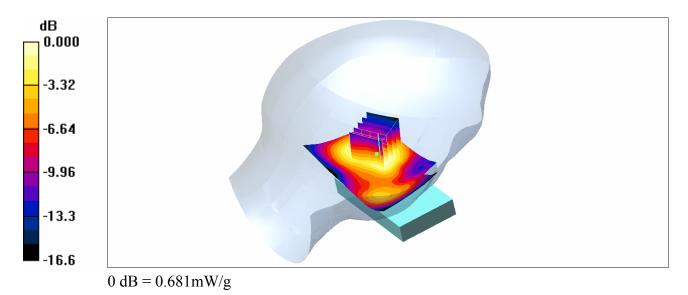
(c) SAR Distribution for EUT in GSM1900 mode measured against the left hand side phantom for the cheek phone position.
