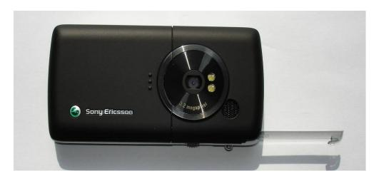
(b) Back of phone with stylus pen partly pulled out.
