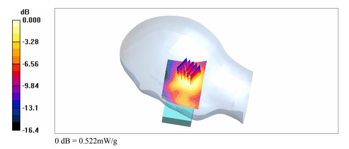
(a) SAR Distribution for EUT in GSM1900 mode measured against the right hand side phantom for the cheek phone position.
