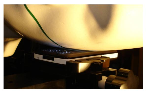
(a) Device on head phantom in the cheek position.
