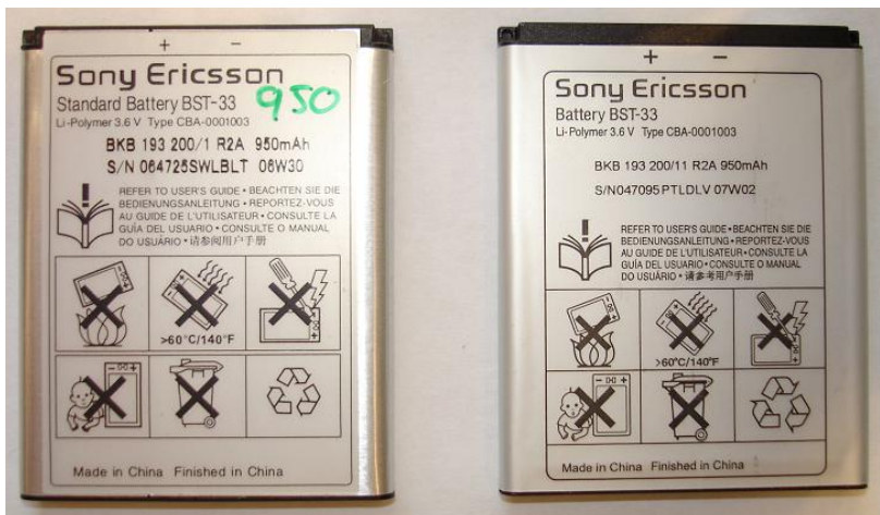
(c) Battery BST-33, type BKB193200/1 (left) and BKB19200/11 (right)
