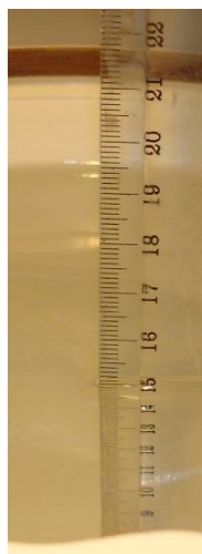
Measured level (152 mm, head section) of 1900 MHz head tissue simulating liquid in phantom.
