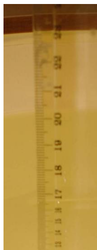
Measured level (167 mm, flat section) of 1900 MHz muscle tissue simulating liquid in phantom
