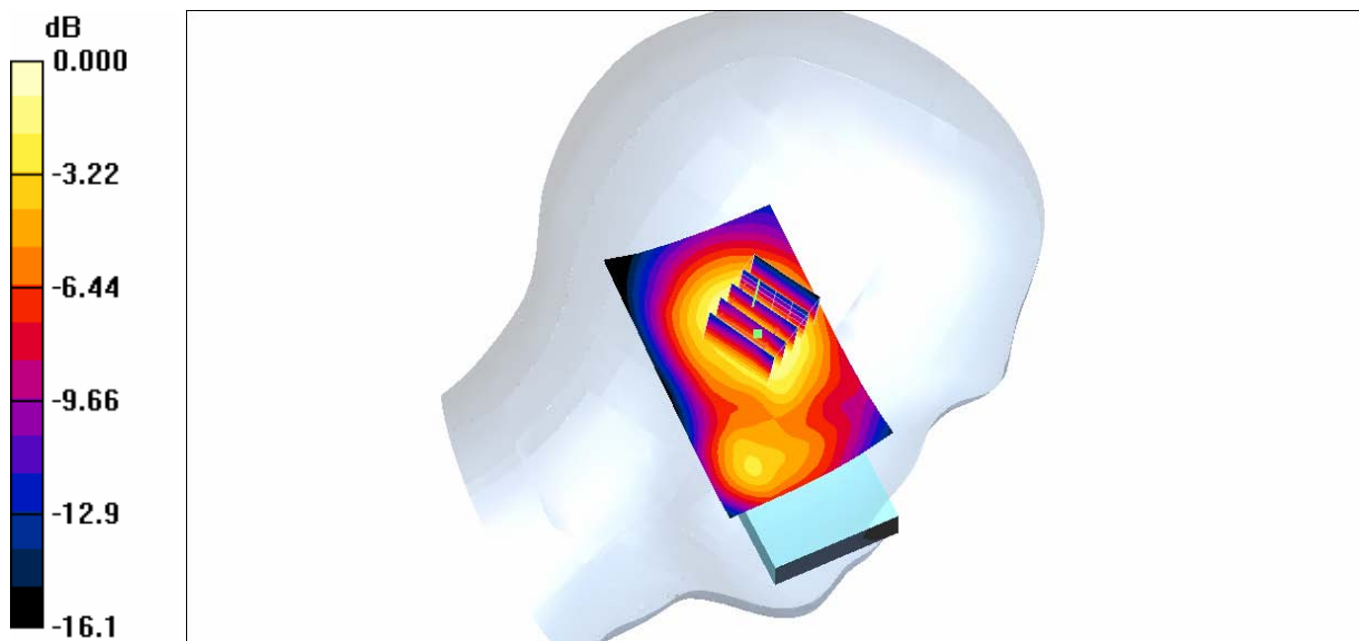
(c) SAR Distribution for mobile phone PY7F3022016 in GSM1900 mode measured against the left hand side phantom for the cheek phone position.
