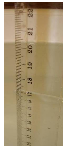
Measured level (172 mm, flat section) of 2450 MHz muscle tissue simulating liquid in phantom
