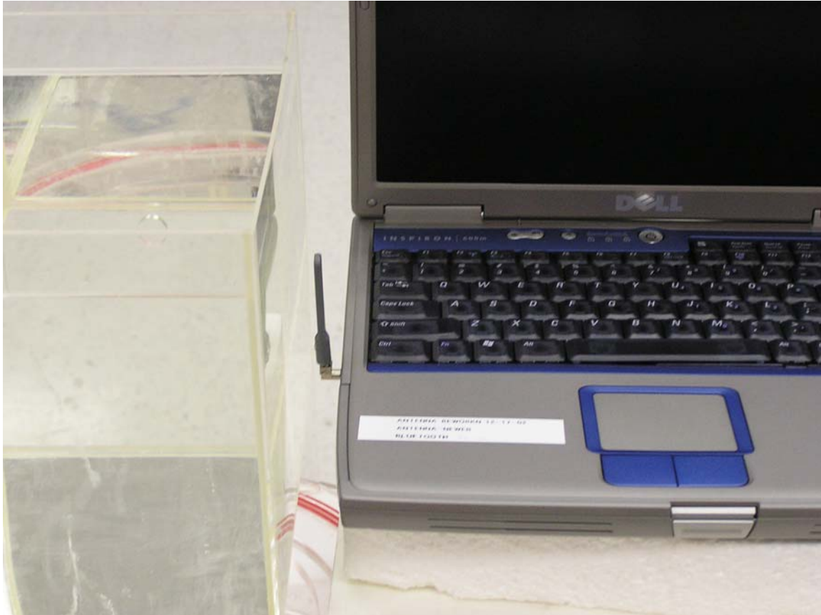
Photo 5. PC #1 bystander antenna vertical
