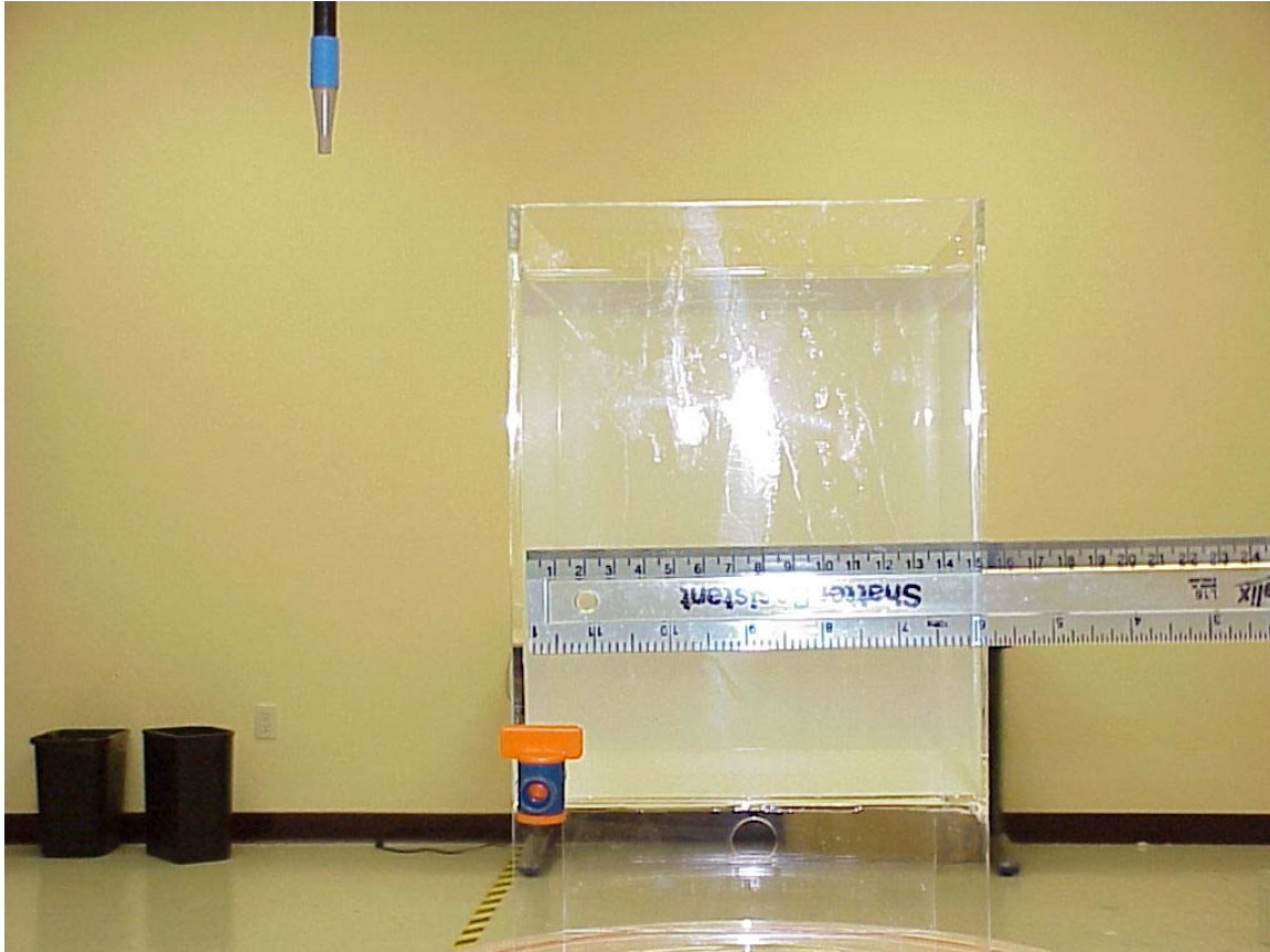
Photo 18. Photo to demonstrate 15 cm Z-axis flat phantom
