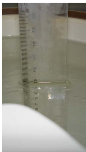
Measured level (151 mm, head section) of 1900 MHz head tissue simulating liquid in phantom.
