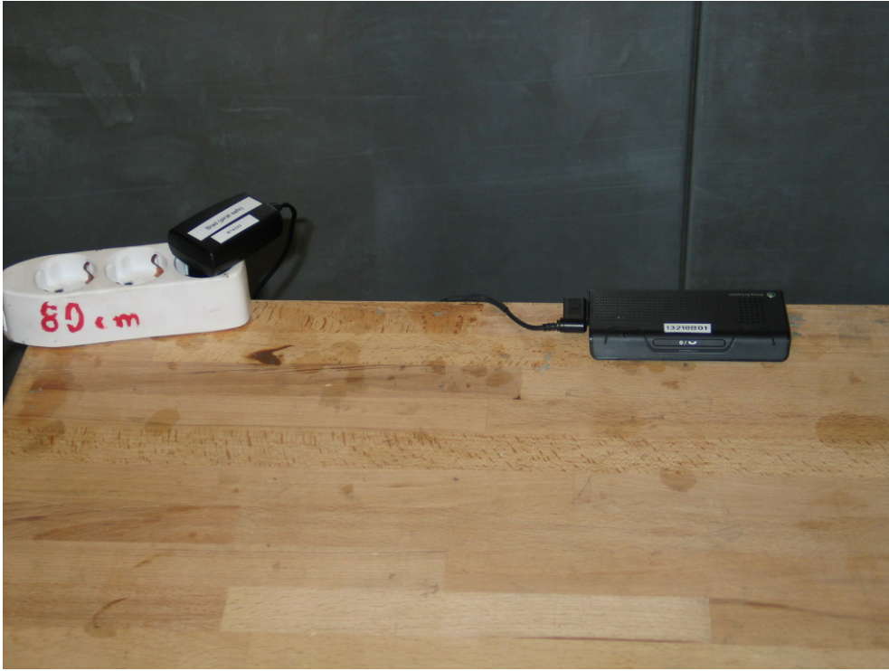
Photo 1: Test setup for conducted measurements at AC port (setup_01 AC)
