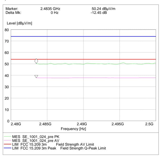
Radiated measurement (higher band edge)
