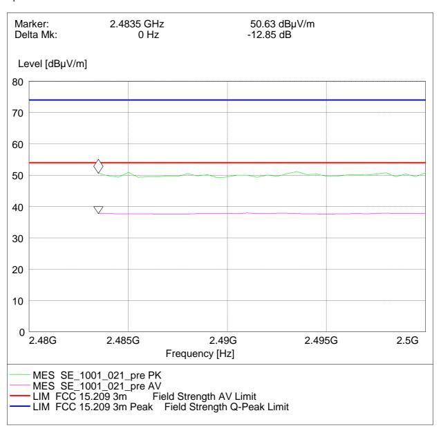
Radiated measurement (higher band edge)
