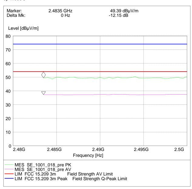
Radiated measurement (higher band edge)
