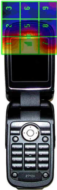
Figure 14 E-Field WD Scan overlay
