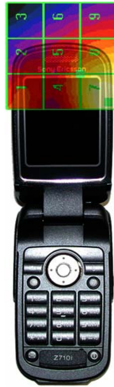
Figure 15 H-Field WD Scan overlay
