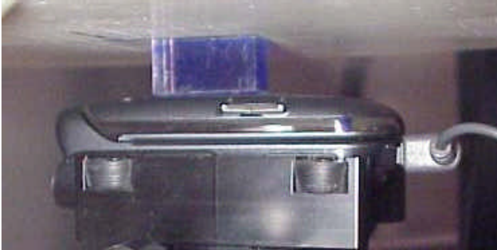
Position with front of device against flat phantom using a 15mm SPACER with hands free accessory.
