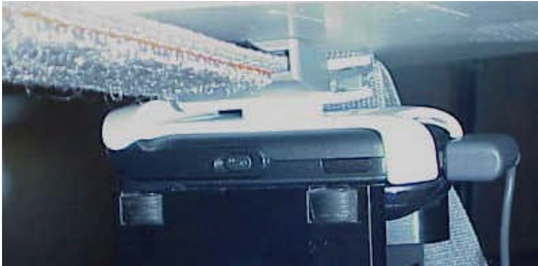
Position with back of device against flat phantom using an IAC60 carry case with hands free accessory.
