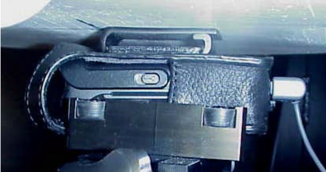
Position with back of device against flat phantom using an ICE26 carry case with hands free accessory.
