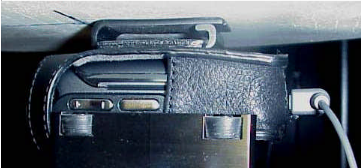
Position with front of device against flat phantom using an ICE26 carry case with hands free accessory.
