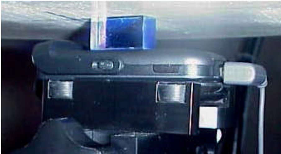
Position with back of device against flat phantom using a 15mm SPACER with hands free accessory.
