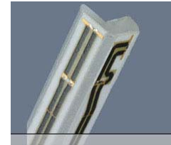
Figure 3 E-field Free-space Probe
