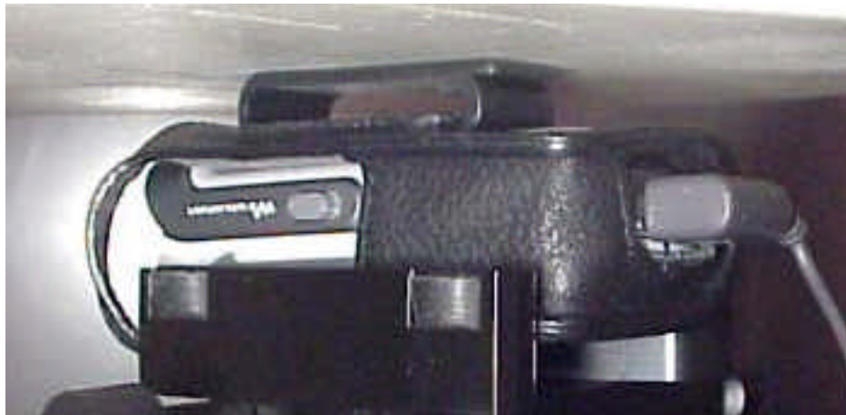
Position with back of device against flat phantom using an ICE26 carry case with hands free accessory.
