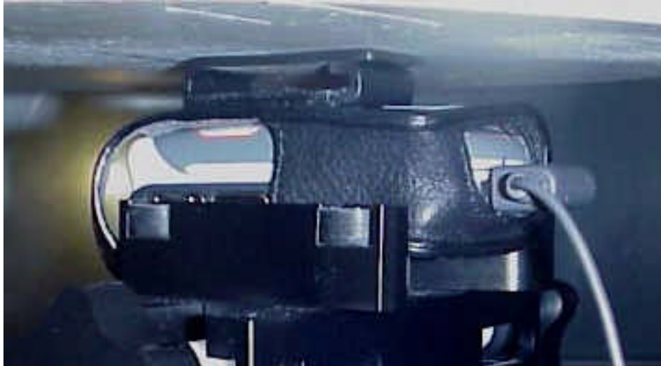
Position with front of device against flat phantom using an ICE26 carry case with hands free accessory.
