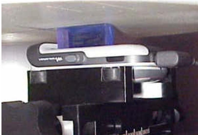
Position with back of device against flat phantom using a 15mm SPACER with hands free accessory.
