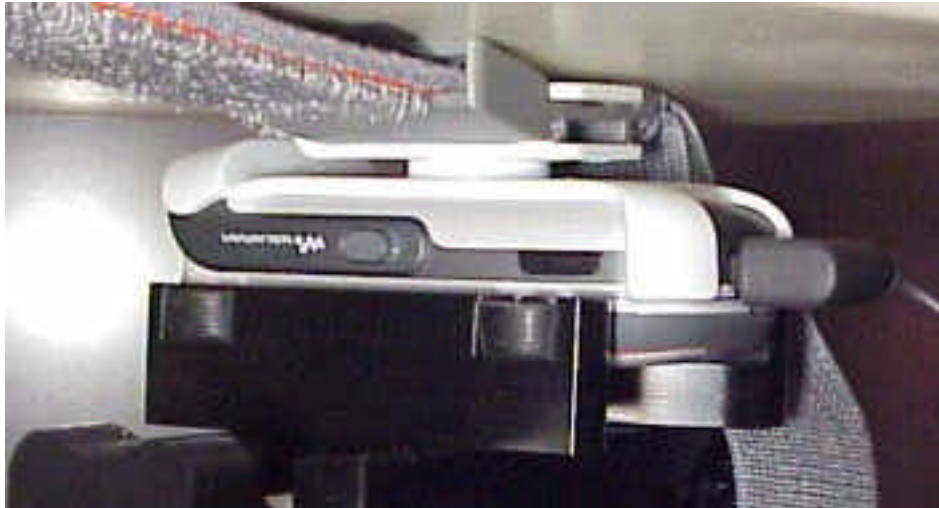
Position with back of device against flat phantom using an IAC60 carry case with hands free accessory.
